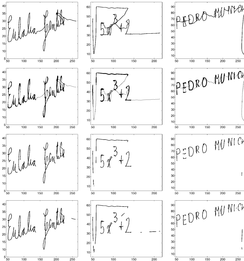
Fig. 13. Point-wise classification results. The first row shows three test sequences. The figures of the second row display each segment of the sequences with a thickness that is proportional to the average of the confidence of the endpoints. Most of the thicker segments corresponds to portions of the trajectory that should be classified as pen down. The third row shows only points of the trajectories that have been classified as pen down using the ink absence confidence measure. The fourth row presents only points that have been classified as pen down by the HMM. We see that there are several segments that appear in areas where there should be no ink trace on the paper. This misclassification is due to a bad measurement of the confidence of ink absence. From the plots of the third and fourth row, it seems that the HMM approach has lower FRR at the cost of a higher FAR.
