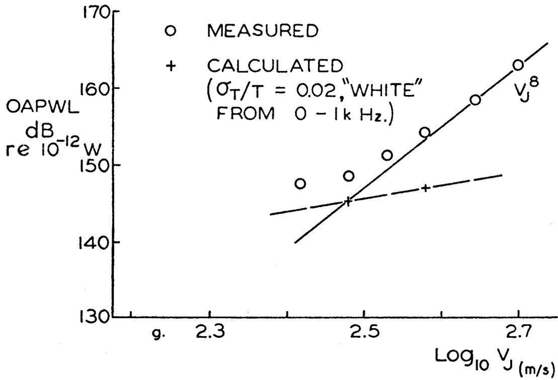
Figure 4. Predicted and measured rear arc overall acoustic power (OAPWL) for the Rolls Royce Olympus 593 (primary nozzle  $0.63 \text{ m}^2$ ).
