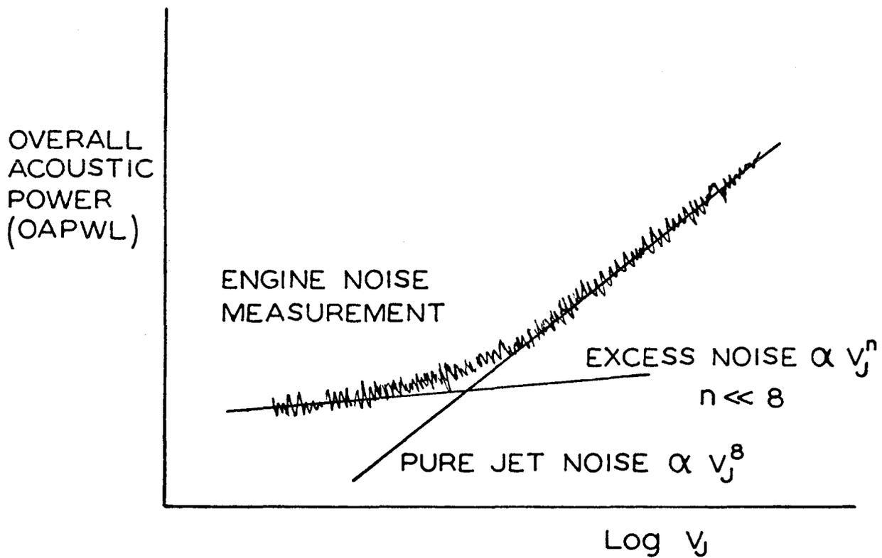
Figure 1. Schematic representation of variation with jet velocity of rear arc noise from a jet engine.
