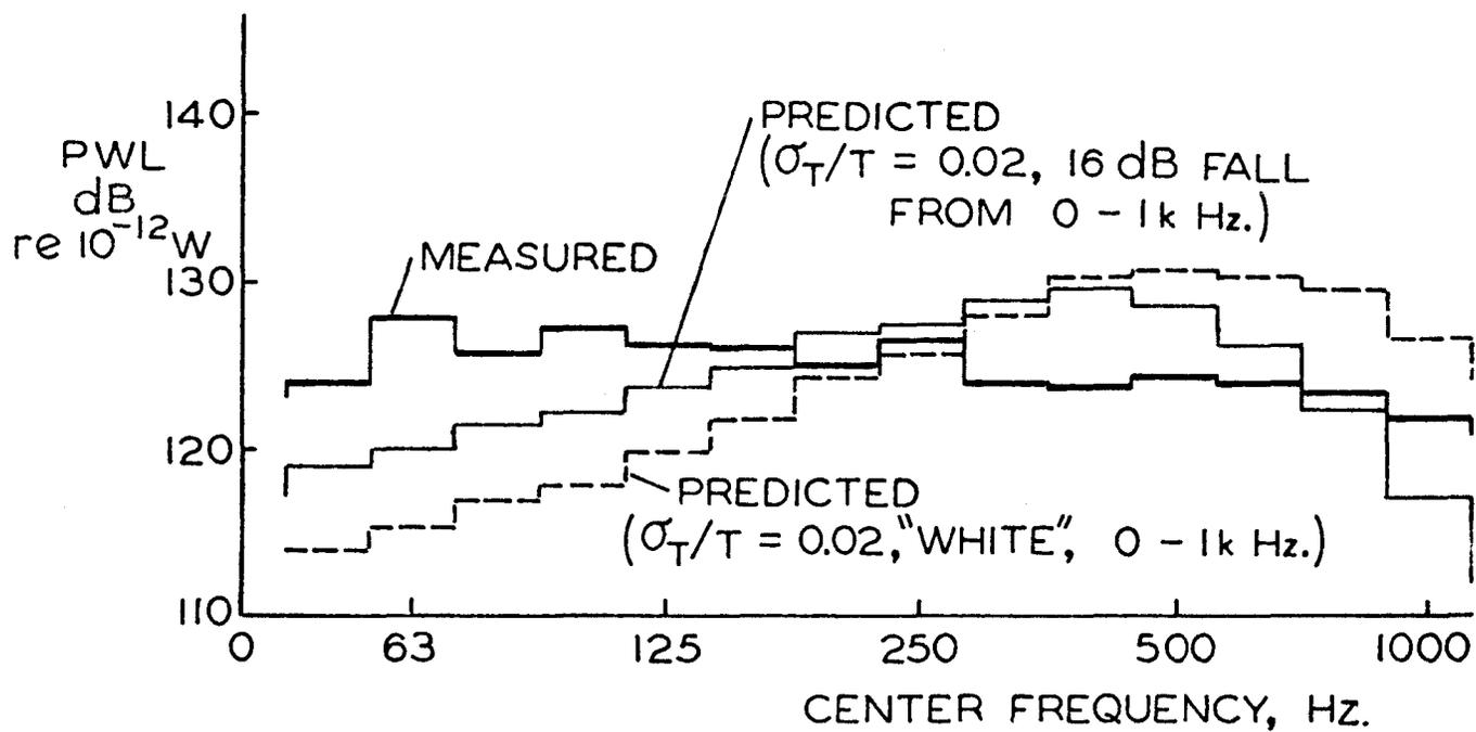
Figure 6. Predicted and measured third octave spectra of rear arc acoustic power for the Rolls Royce Spey 512 (jet velocity 216 m/s).
