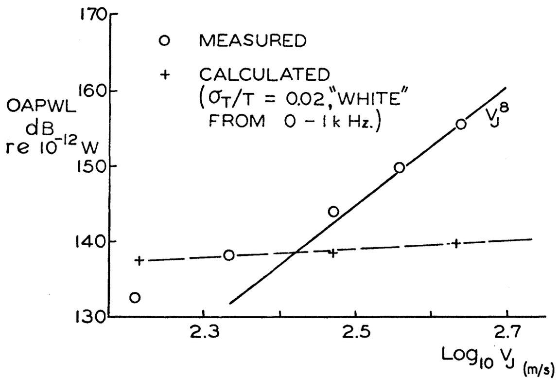
Figure 3. Predicted and measured rear arc overall acoustic power (OAPWL) for the Rolls Royce Spey 512.
