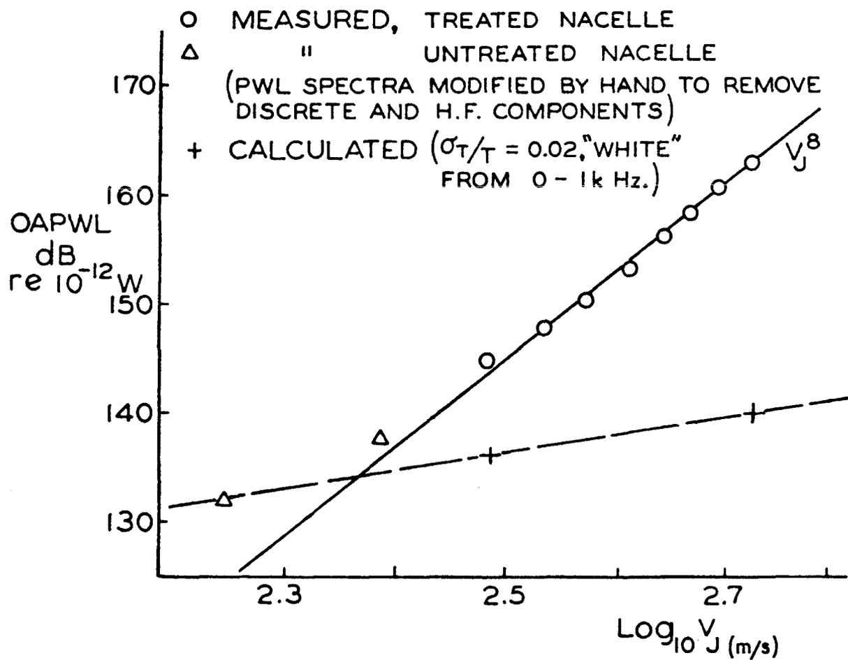
Figure 5. Predicted and measured rear arc overall acoustic power (OAPWL) for the Pratt and Whitney JT8D-9.
