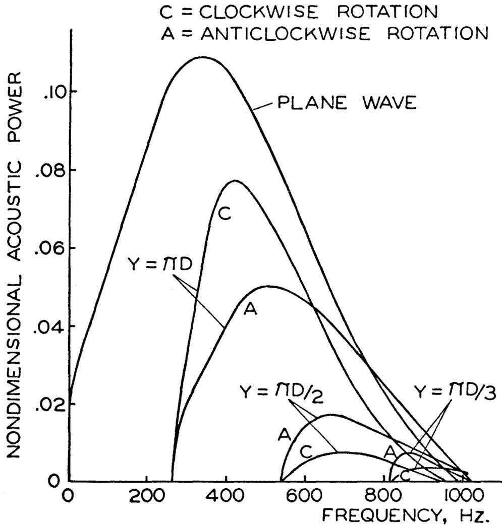
Figure 2. Non-dimensional acoustic power for the Rolls Royce Spey produced by each Fourier component of temperature fluctuation.
