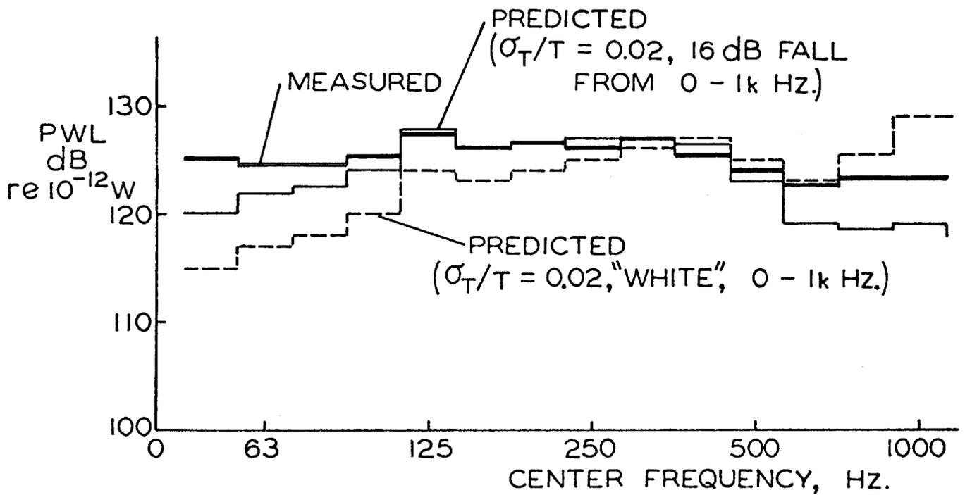
Figure 7. Predicted and measured third octave spectra of rear arc acoustic power for the Pratt and Whitney JT8D-9 (jet velocity 275 m/s).
