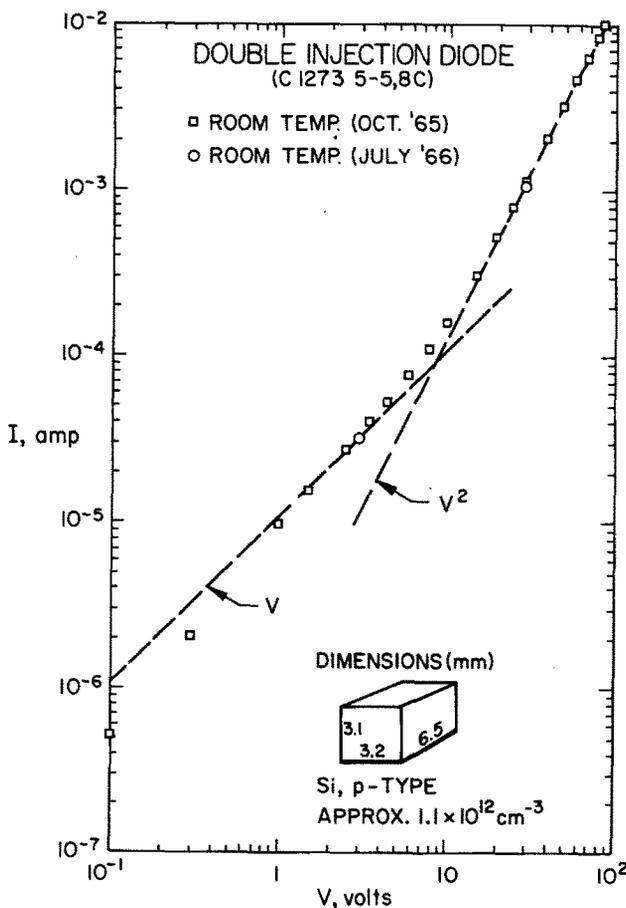
Fig. 1. V-I characteristic of double-injection diode at room temperature. The circles indicate the two operating points for which noise measurements are reported.
