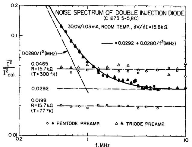
Fig. 2. Noise spectra of double-injection diode (30 V/1.03 mA, room temperature), of a 15.7 kΩ resistor at room temperature and immersed in liquid nitrogen. The spectrum of the diode is the sum of  $1/f^2$  excess noise and a white component (dashed lines).
