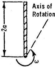
$$T_1 = \frac{9}{16} \rho \pi a^4 \omega^2, \quad \text{as in Equation [106b]'} \\ \text{with } \beta = 1,$$
