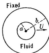
$$T_1 = \frac{1}{2} \rho \pi a^2 U^2 \frac{b^2 + a^2}{b^2 - a^2}, \quad \text{as in Equation [104f]}$$
