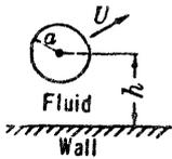
$$T_1 = \frac{1}{2} \rho \pi a^2 U^2 \left( 1 + \frac{a^2}{2h^2} \dots \right), \quad \text{as in Equation [95g]}$$
