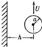
$$T = \frac{\pi}{3} \rho a^3 \left( 1 + \frac{3}{16} \frac{a^3}{h^3} + \dots \right) U^2, \quad \text{as in Equation [130a]}$$
