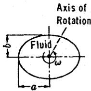
$$T_1 = \frac{1}{8} \rho \pi a b \frac{(a^2 - b^2)^2}{a^2 + b^2} \omega^2, \quad \text{as in Equation [105m],}$$
