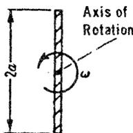
$$T_1 = \frac{1}{16} \rho \pi a^4 \omega^2, \quad \text{as in Equation [106a'],}$$
