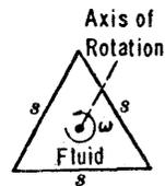
$$T_1 = \frac{1}{80\sqrt{3}} \rho s^4 \omega^2, \quad \text{as in Equation [103k],}$$
