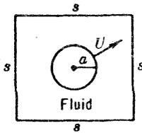
$$T_1 = \frac{1}{2} \rho \pi a^2 U^2 \left( 1 + 6.88 \frac{a^2}{s^2} \dots \right),$$
