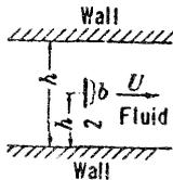
$$T_1 = \frac{1}{2} \rho U^2 \frac{\pi b^2}{4} \left( 1 + \frac{\pi^2 b^2}{24 h^2} \dots \right), \quad \text{as in Equation [651]}$$
