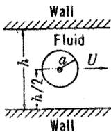
$$T_1 = \frac{1}{2} \rho \pi a^2 U^2 \left[ 1 + \frac{2}{3} \left( \frac{\pi a}{h} \right)^2 + \dots \right], \quad \text{as in Equation [46q]}$$
