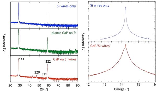
**Figure 6. X-ray diffraction measurements of GaP/Si and Si samples. Top:  $\omega$ - $2\theta$  scans. Bottom: rocking curves.**
