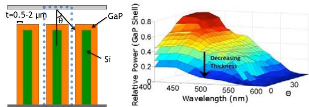
**Figure 1. Simulated two-dimensional GaP/Si "grating" absorption. The simulation unit cell is outlined by the dotted box.**
