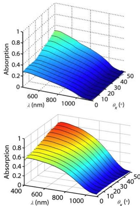
**Figure 7. Optical absorption of peeled-off wire arrays: Top: Si wires only, Bottom: GaP-coated Si wires.**
