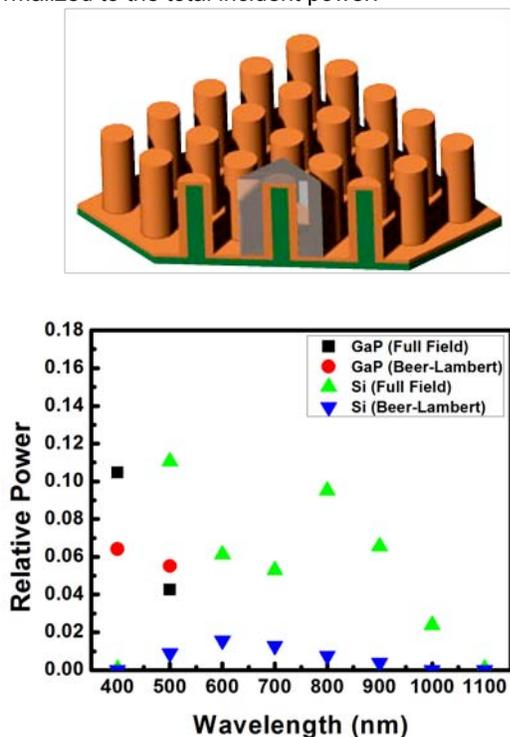
**Figure 2. Normal incident GaP/Si wire array absorption. The simulation unit cell is outlined in the top diagram.**
