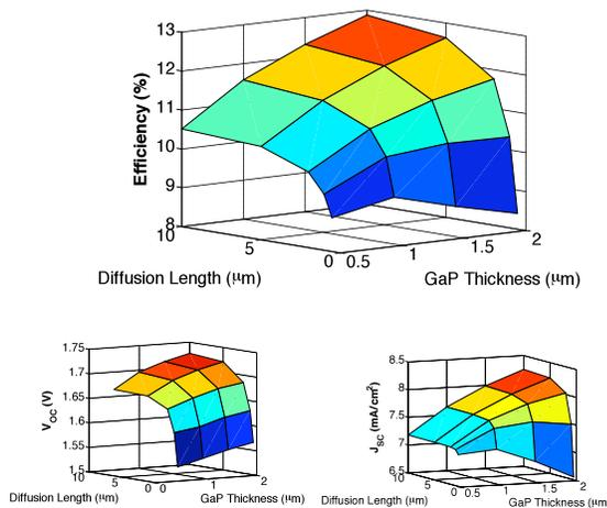
**Figure 4. Simulated GaP/Si wire array efficiency, open circuit voltage ( $V_{oc}$ ), and short circuit current ( $J_{sc}$ ) contour plots assuming Beer-Lambert absorption**
