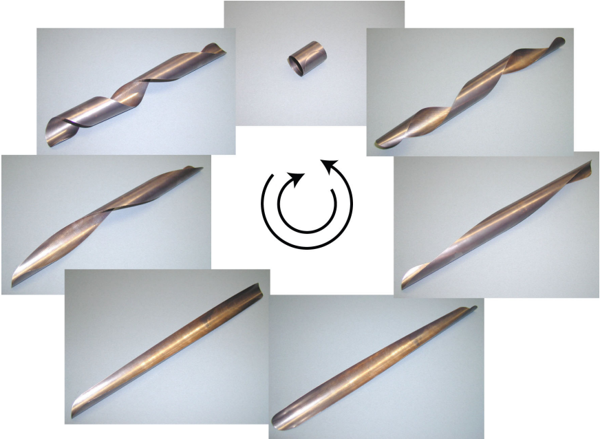
Figure 1. A series of different configurations of the same zero-stiffness shell structure. In each configuration, the shell is held in place by no more than the friction with the underlying surface. The shell can be transformed between configurations in both directions, clockwise and anticlockwise. The analytical model in Section 2 predicts that the shell will, in each case, be wrapped around an underlying cylinder (see Figure 3 ) of constant radius, and it can be seen that this is the case here.
