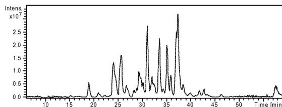
**Figure 6** Separation of BSA Digest using commercial HPLC system.
