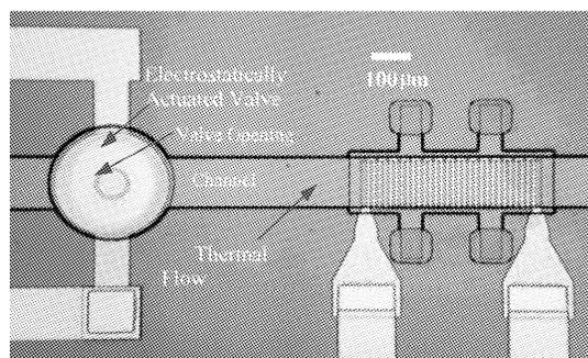
**Figure** Fabricated mass flow controller
