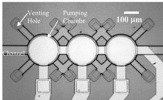
**Figure 4** Fabricated micro peristaltic pump.
