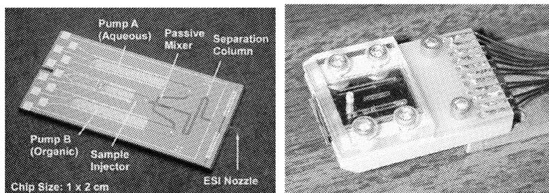
**Figure 5** A photograph of the fabricated HPLC lab-on-a-chip. The picture on the right is a fully packaged HPLC system that can be connected directly to mass spectrometers through electrospray ionization (ESI).
