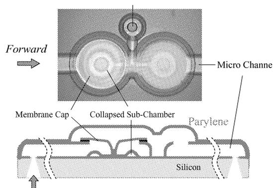
**Figure 2** a surface-micromachined normally closed in-channel check valve using 5-layers of Parylene.
