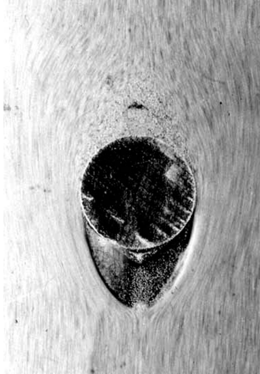
Figure 13.1. Long exposure photograph of the downward flow of sand around a circular cylinder. Reproduced with the permission of R.H.Sabersky.
