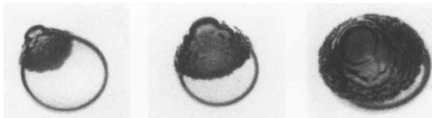
Figure 4.8. Typical photographs of a rapidly growing bubble in a droplet of superheated ether suspended in glycerine. The bubble is the dark, rough mass; the droplet is clear and transparent. The photographs, which are of different events, were taken 31, 44, and 58 \mu\text{s} after nucleation and the droplets are approximately 2mm in diameter. Reproduced from Frost and Sturtevant (1986) with the permission of the authors.
