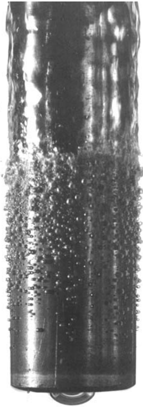
Figure 6.5. The evolution of convective boiling around a heated rod, reproduced from Sherman and Sabersky (1981) with permission.
