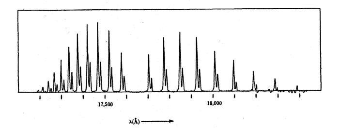
FIGURE 5-4 The first overtone band of HCl taken on a Cary model 14 spectrometer. The strong set of lines is from HCl<sup>35</sup>; the weak set is from HCl<sup>37</sup>. The unequal spacings between lines show the effects of vibration-rotation coupling. Each division on the wavelength scale equals 100 Å.
