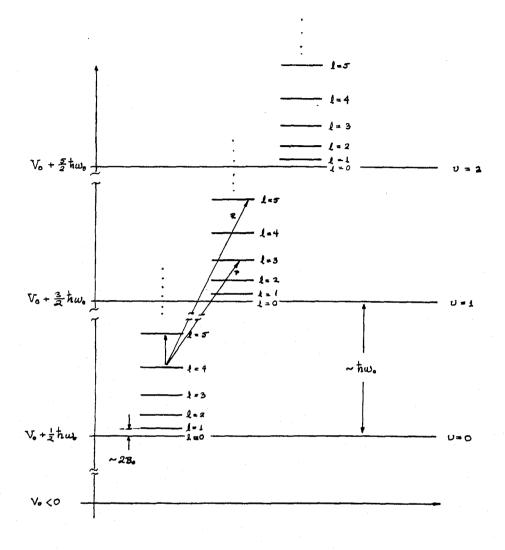
Vibrational-rotational absorption transitions of a diatomic molecule.
