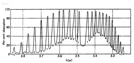
F1G. 9-13. The absorption spectrum of HCl vapor in the near infrared. [After Imes, Astrophys. J., 50, 251 (1919).]
