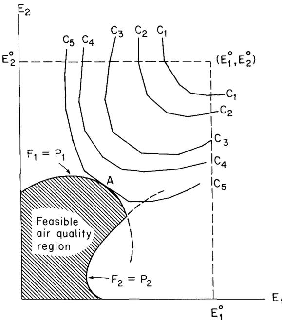
**Figure 9.5** Iso-cost lines in the plane of emission levels of two pollutants,  $E_1$  and  $E_2$ , showing a feasible region of air quality defined by the curves  $F_1(E_1, E_2) \leq P_1$  and  $F_2(E_1, E_2) \leq P_2$ .
