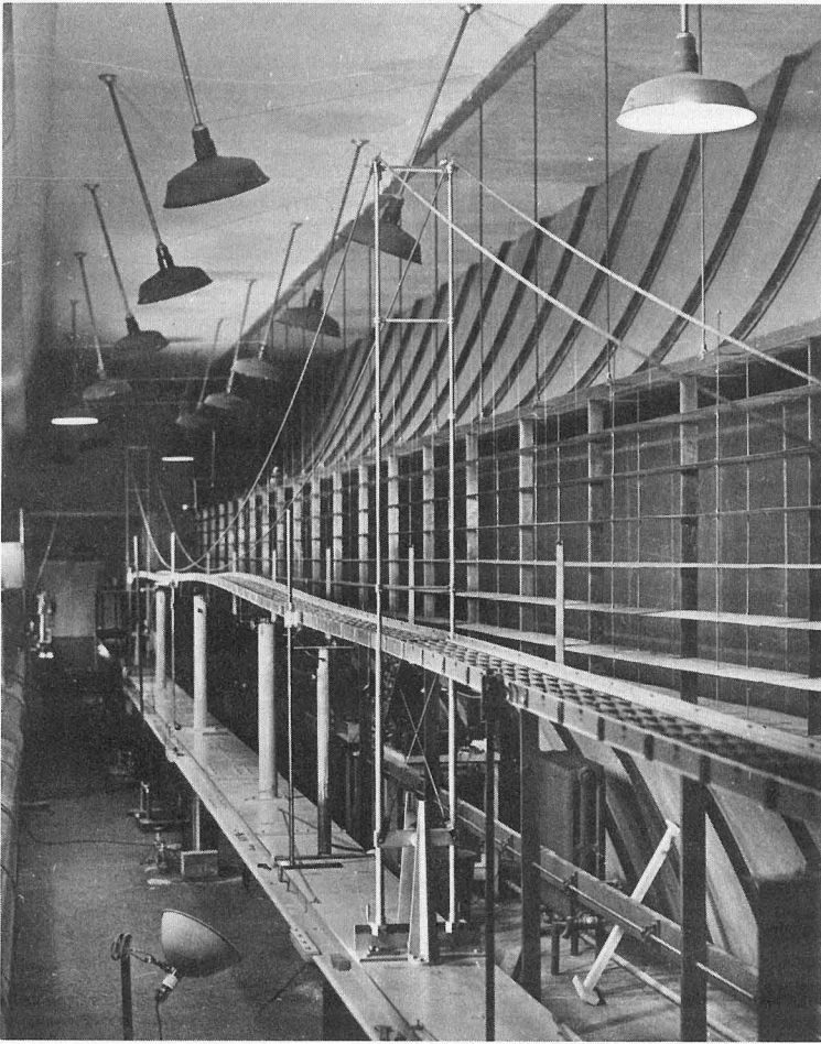
A 1:50 scale model of the Tacoma Narrows Bridge, assembled for tests in a specially designed wind tunnel at the University of Washington. Von Kármán, who was called in as a consultant to investigate the bridge's failure, showed that the torsional oscillations could be explained by his own 1911 work on vortex patterns.
