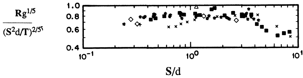
Figure 4.3.3b The runup number variation with the stroke of the generator. Type R waves.
