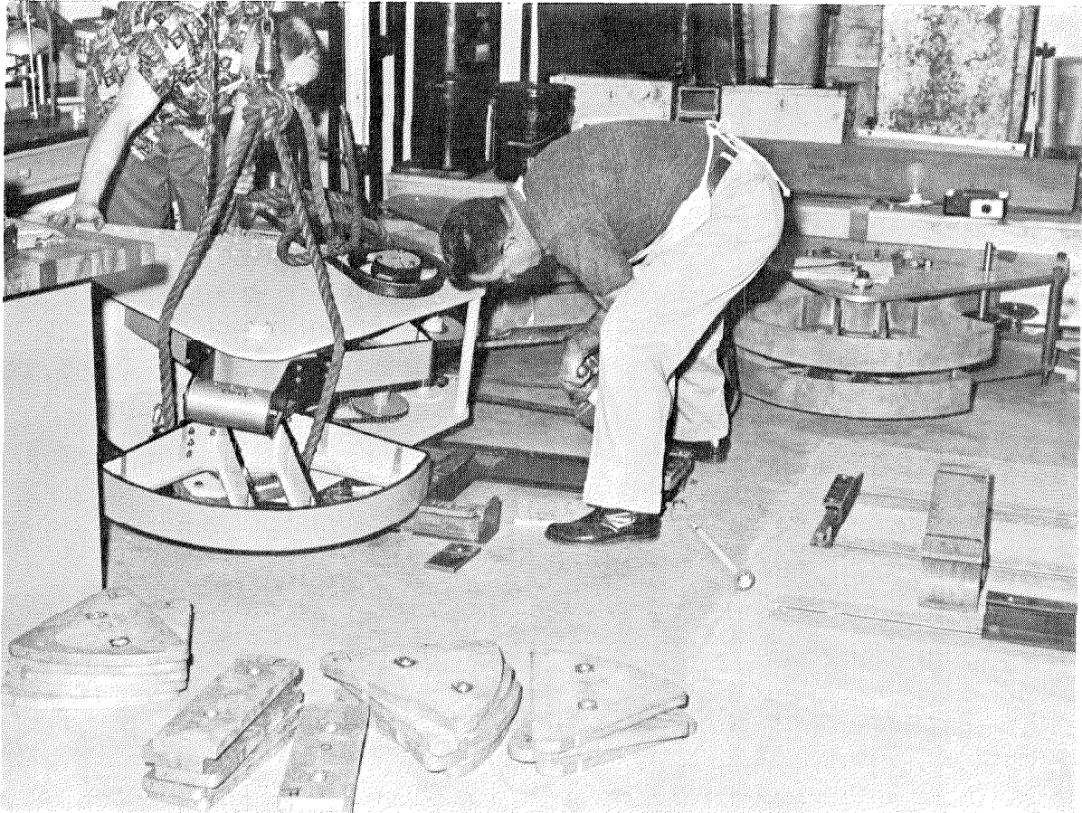
Fig. 3. Vibration Exciter Unit Being Installed in Laboratory
