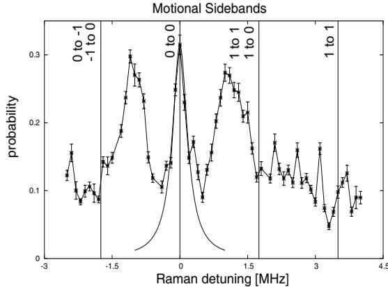
**FIGURE 3. Motional Raman sidebands for one trapped atom.** The atom is initially prepared as described in Fig. 2 and in the text. We drive the transition ( $F = 3, m_F = 0$ )  $\leftrightarrow$  ( $F = 4, m_F = 0$ ) with  $\Omega_E = 200$  kHz for various Raman detunings  $\delta$ . The detuning  $\delta = 0$  is chosen to coincide with the transition between  $m_F = 0$  levels; the frequencies of other (suppressed) transitions between Zeeman levels are indicated.
