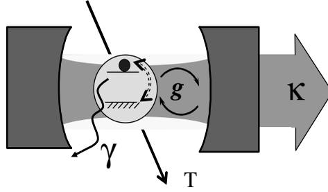
**FIGURE 1. Characteristic parameters of atom, cavity, and environment:**  $\kappa$ , the rate of decay of the cavity field;  $\gamma$ , the rate at which the atomic dipole radiates into modes other than the cavity field mode;  $T$ , the transit time of an atom through the cavity mode; and  $g$ , the rate of coherent atom-field coupling. Strong coupling requires that  $g/(\gamma, \kappa, \frac{1}{T}) \gg 1$ .
