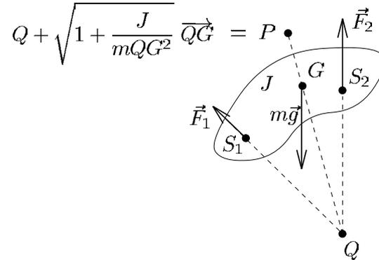
Figure 3: Planar rigid solid controlled by two body fixed forces.
