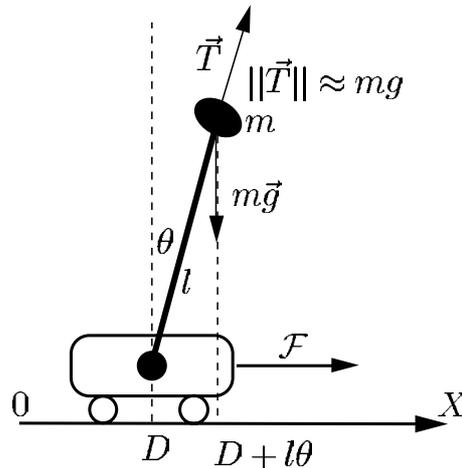
Figure 1: Inverted pendulum.
