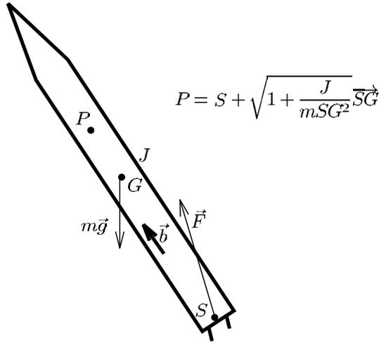
Figure 4: a rocket and its flat output  $P$ .
