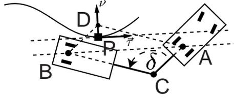
Figure 12: geometric construction with the Frénet frame.
