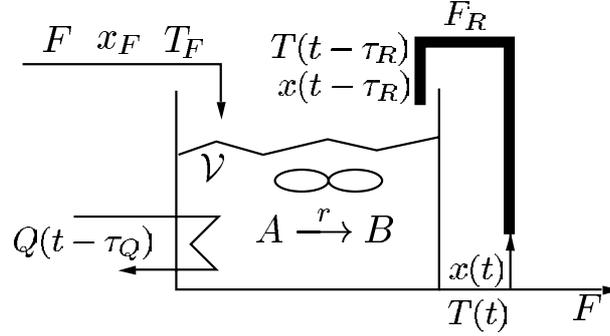
Figure 17: A chemical reactor with a recycle loop.
