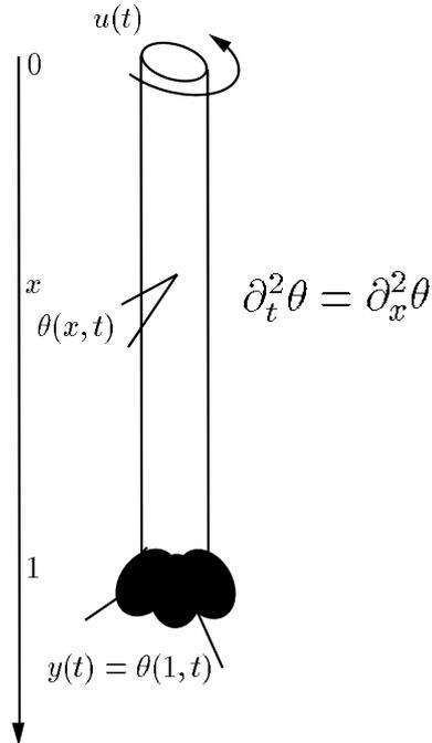
Figure 24: torsion dynamics of a drilling system.
