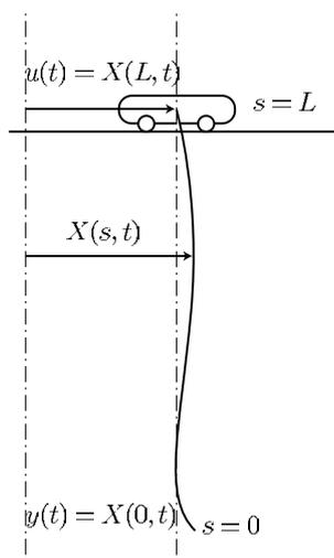
Figure 15: the homogeneous chain without any load.
