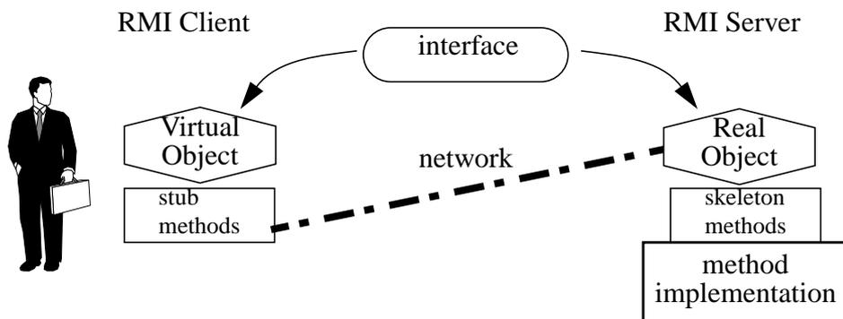
**Figure 2.** Client-Server communication through Java RMI (Remote Method Invocation). Each shared object has an interface, common to client and server sides, that defines what methods are available. The client can invoke methods on the object, but these are executed on the server where the object actually resides.
