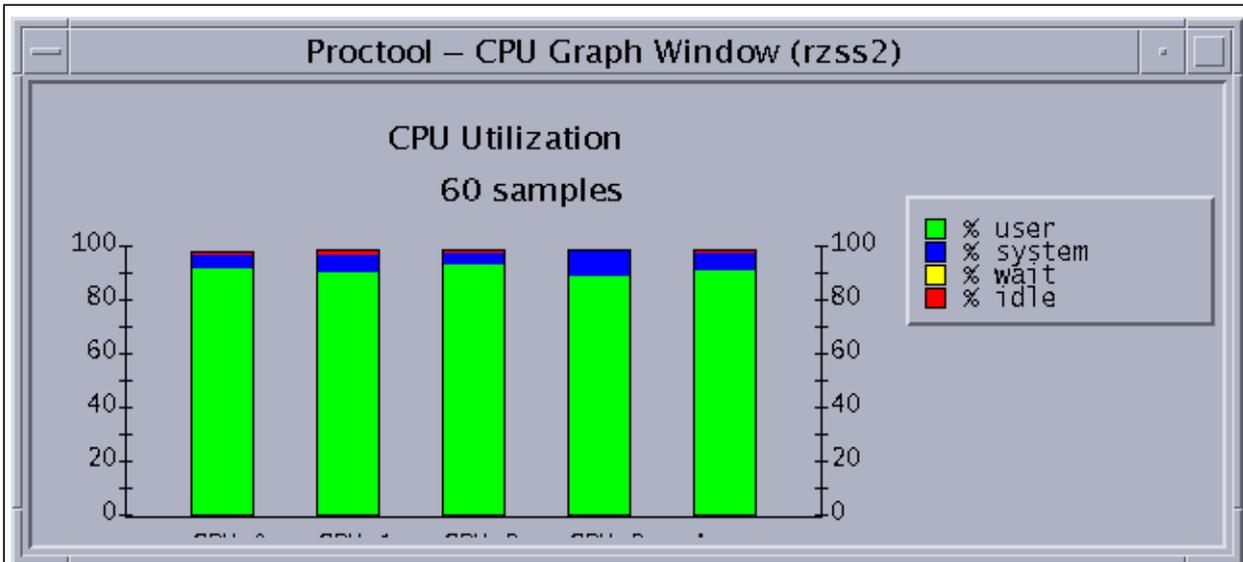
**Figure 9.** Processor utilization for the 4-processor Sun E450 running JParNss. This screenshot is obtained from the Solaris tool *proctool*. The bars from left to right denote CPU numbers 0 to 3, the rightmost bar shows the average load of the CPUs. It is important that the thread scheduler generates a full computational load for all processors. If the number of threads is too small or threads of highly different computational load have been produced, parallel efficiency is reduced.
