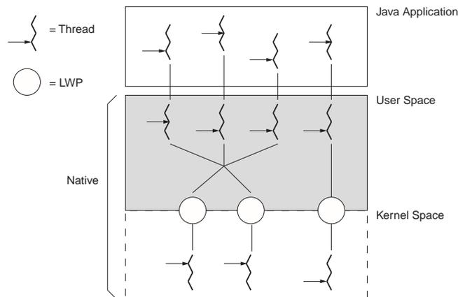
**Figure 6.** The many-to-many model (many user-level threads to many kernel-level threads) avoids many of the limitations of the one-to-one model, while extending multithreading capabilities even further. The many-to-many model, also referred to as the two-level model, minimizes programming effort while reducing the cost and weight of each thread.
