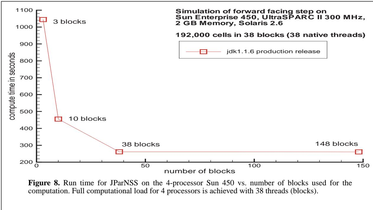
times as the number of blocks of the multiblock grid is varied. Here the number of active threads is the same as the number of blocks. As blocks are split, we have more threads than processors, so that each processor has enough work to do: the computational efficiency increases because the load-balance between the four processors improves. For a much larger number of blocks, however, the thread overhead becomes larger than the
