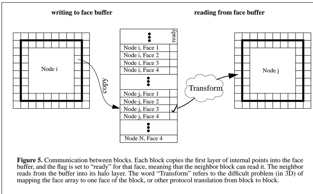
**Figure 5.** Communication between blocks. Each block copies the first layer of internal points into the face buffer, and the flag is set to “ready” for that face, meaning that the neighbor block can read it. The neighbor reads from the buffer into its halo layer. The word “Transform” refers to the difficult problem (in 3D) of mapping the face array to one face of the block, or other protocol translation from block to block.
