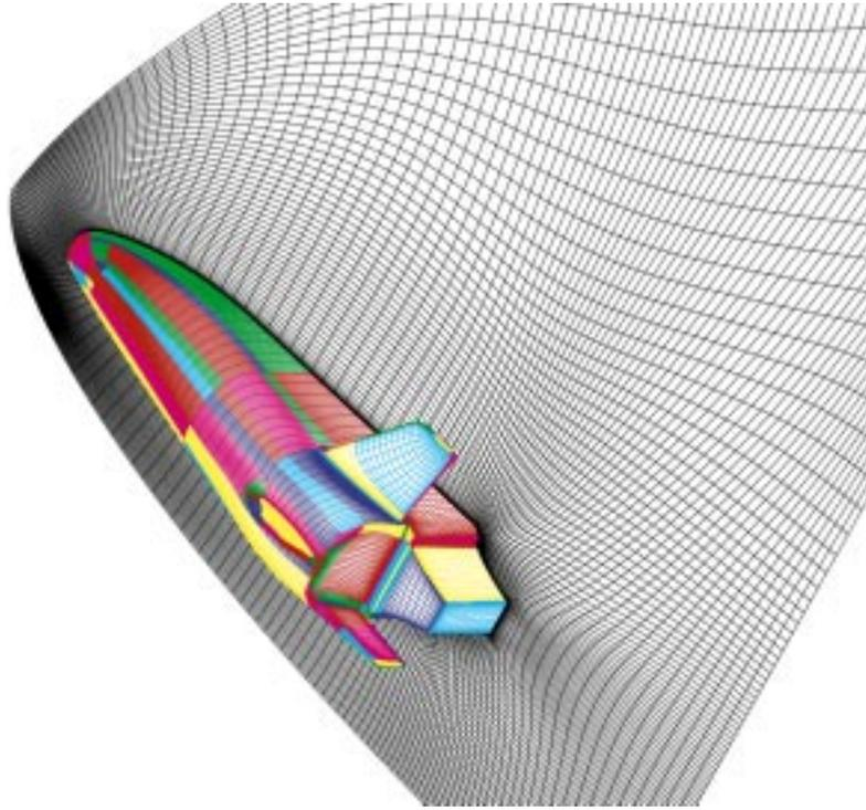
**Figure 1:** A multiblock grid for the X-33 vehicle. Each block is run in its own thread. Grids may have thousands of blocks, and thus the OS has to create the corresponding number of threads and is also responsible for starting and stopping all threads.
