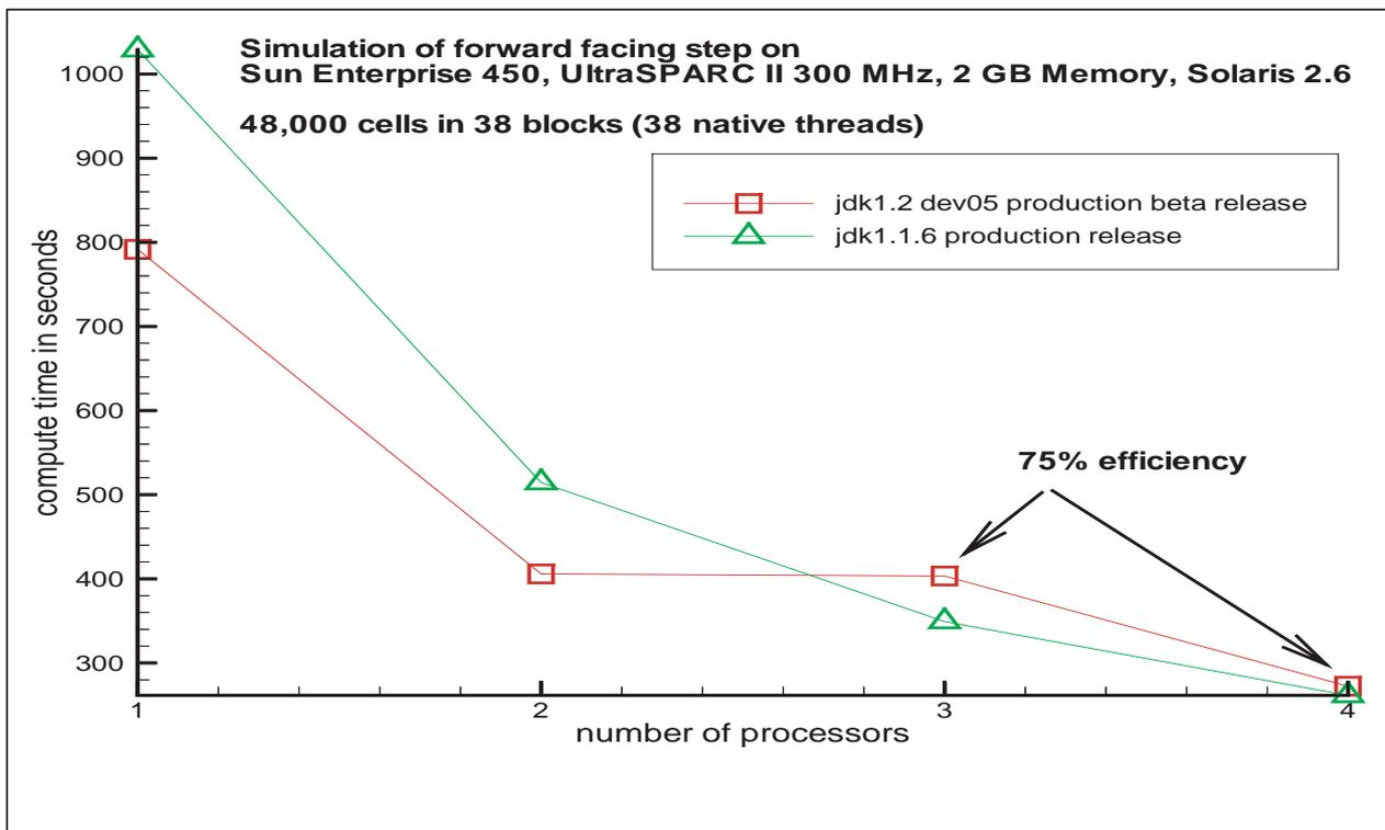
**Figure 10.** Run time for JParNss on the 4-processor Sun 450 vs. number of processors. The 38 block grid comprising 48,000 cells was used for the simulations. The figure shows a substantial speedup for the 1 and 2 processor configurations for JDK1.2 over JDK1.1.6. However, when 3 and 4 processors are used, JDK 1.2 does not scale properly and parallel efficiency is lost.
