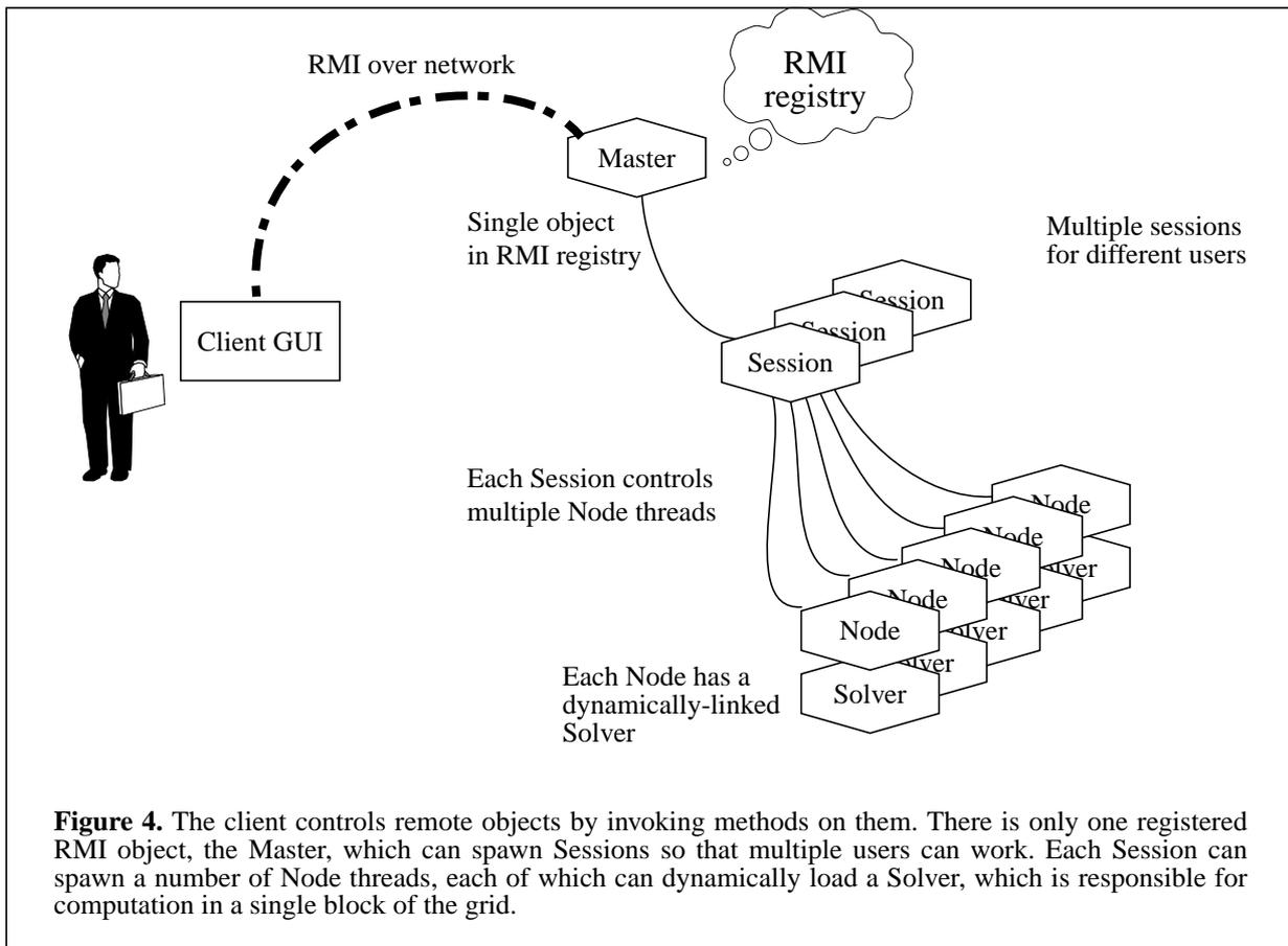
**Figure 4.** The client controls remote objects by invoking methods on them. There is only one registered RMI object, the Master, which can spawn Sessions so that multiple users can work. Each Session can spawn a number of Node threads, each of which can dynamically load a Solver, which is responsible for computation in a single block of the grid.
