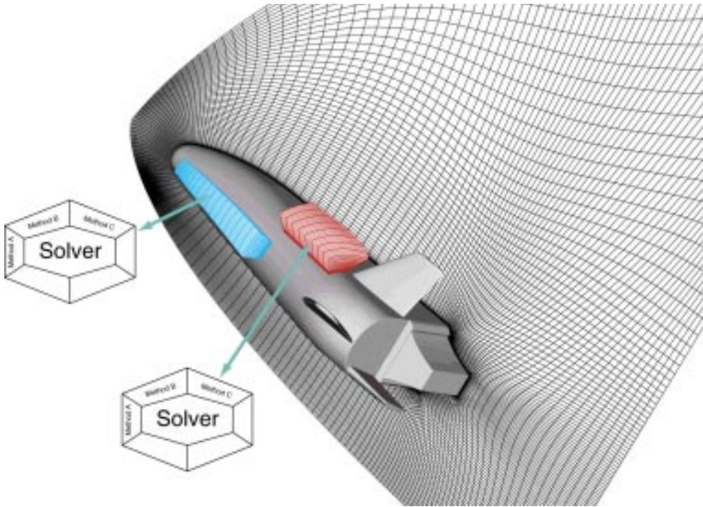
**Figure 3.** Every solver object contains the data of and the numerics for one block. The solver class is sent from the client to the server that is, different users may use different solvers.
