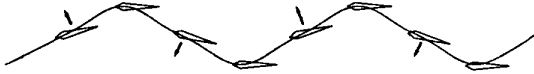
Figure 2: A “cartoon” of carangiform swimming consisting of snapshots of the tail as the fish swims from left to right. The arrows indicate lift forces acting on the tail. The fish body is removed for clarity.
