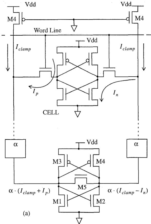
Figure 4. The bitline structure and the offset definitions.
