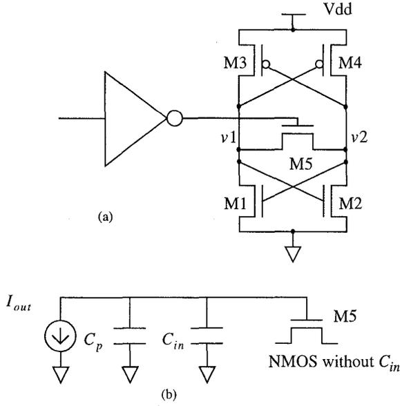
Figure 2. Equivalent circuit for the equilibrating device.
