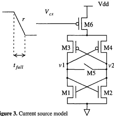
**Figure 3.** Current source model where  $t_f$  is the fall time of  $V_{cs}$ . From the above equation for  $t = t_f$
