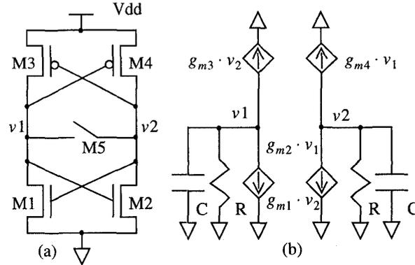
Figure 1. The simplified model for the sense amplifier.
