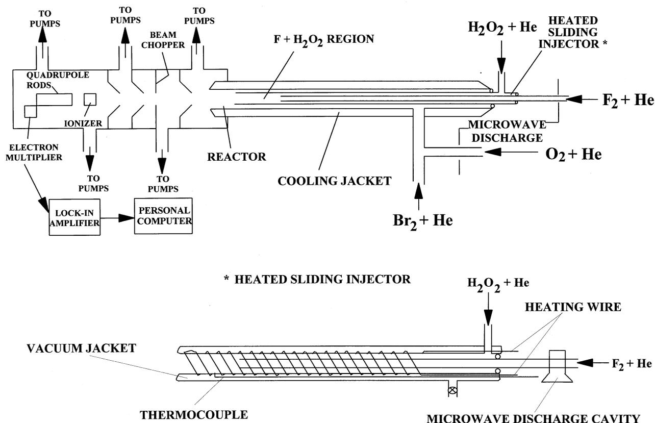
Fig. 1 Schematic diagram of the experimental apparatus for the study of BrO + HO<sub>2</sub> kinetics
