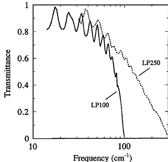
Fig. 2. Plot of the in-band transmittance of a 360- $\mu$ m-thick sample from a LP100 filter (solid curve) and from a 245- $\mu$ m-thick sample from a LP250 filter (dotted curve).
