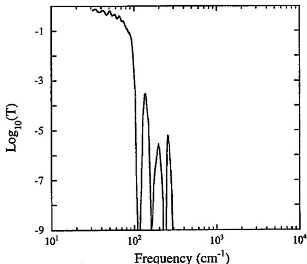
Fig. 4. Calculated transmittance of a low-pass filter stack consisting of two 360- $\mu\text{m}$  sheets of the LP100 component and one 245- $\mu\text{m}$  sheet of the LP250 component. The transmittance is  $< 10^{-9}$  for  $\nu > 300 \text{ cm}^{-1}$ .
