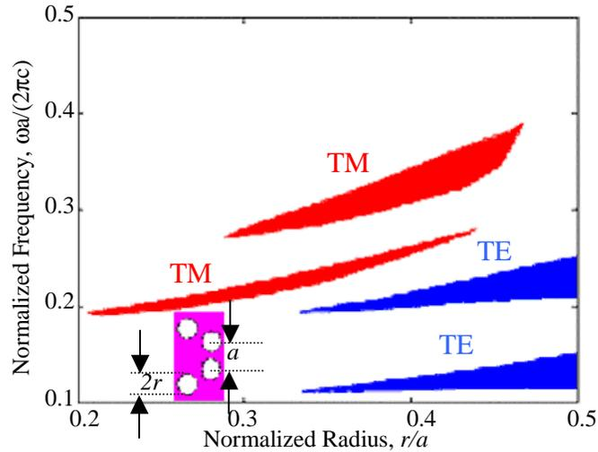
Fig. 1. Maps of photonic bandgap for TE (electric field perpendicular to the computation plane) and TM polarizations in a two-dimensional hexagonal-lattice structure of air cylinders in GaAs ( $\epsilon=12.96$ ) as functions of the ratio  $r/a$ .
