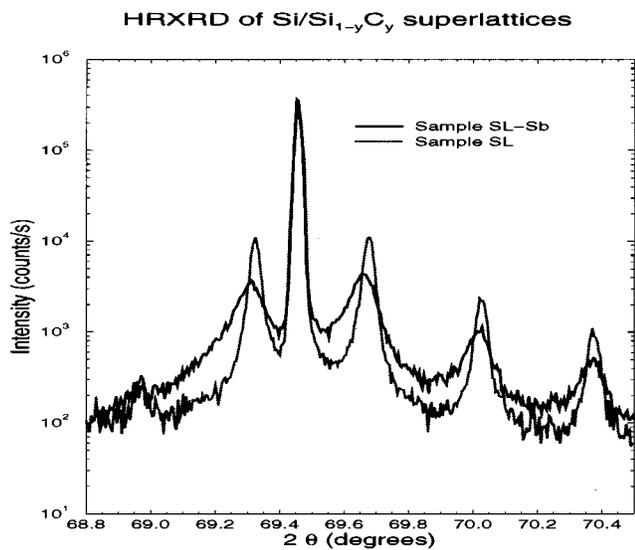
FIG. 4. HRXRD of a 15 period Si/Si<sub>0.97</sub>C<sub>0.03</sub> superlattice grown by standard MBE (sample SL) and by Sb assisted MBE (sample SL-Sb). The sample SL superlattice peaks are sharper than those of sample SL-Sb. This is probably due to the Si/Si<sub>0.97</sub>C<sub>0.03</sub> interfaces being less sharp in the SL-Sb sample (as observed in the cross-sectional TEM micrographs, Fig. 3) or a higher density of stacking faults in sample SL-Sb as compared to sample SL.
