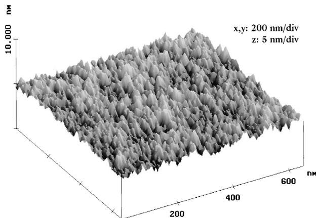
FIG. 5. AFM micrograph of the top layer (Si<sub>0.97</sub>C<sub>0.03</sub>) of a 15 period Si/Si<sub>0.97</sub>C<sub>0.03</sub> superlattice grown by standard MBE (sample SL). The features are on the order of 1.4 nm tall and 40 nm on the side. These surface features apparently give rise to the spotty RHEED pattern observed [see Fig. 1(c)] and the variation in thickness seen in the TEM (see Fig. 3).
