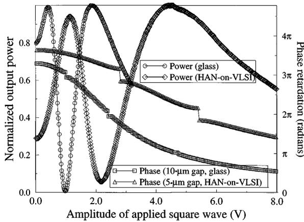
Fig. 2. Electro-optic characteristics at 632.8 nm of a transmissive HAN cell with a 10- $\mu\text{m}$  gap and a reflective HAN-on-VLSI sample with a 5- $\mu\text{m}$  gap. Both cells were filled with Merck E7. Note that the entire amplitude-modulation range of the HAN-on-VLSI device is spanned by the 1.1-V amplitude interval between 1.1 and 2.2 V.
