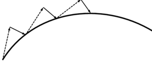
FIGURE 2. Sketch of the numerical implementation for computing the VSF. Solid curve, solution of the VSF; dashed arrow, prediction step (3.4); solid arrow, correction step (3.5).
