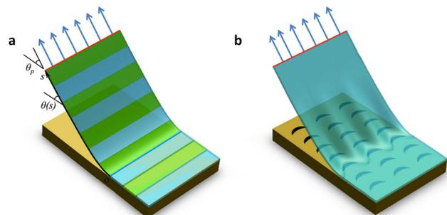
FIG. 1 (color online). Peeling of adhesive tapes with (a) elastic and (b) adhesive heterogeneities.
