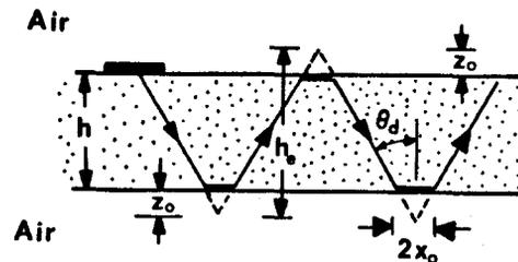
Fig. 6 Effective thickness: ray picture,  $h_e = h + 2z_0$ .
