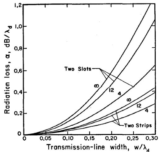
Fig. 7 Theoretical losses for lines with a strip or slot spacing equal to 1/3 the total width. The dielectric constants are indicated. The substrate thickness is assumed to be much greater than  $\lambda_d$ .
