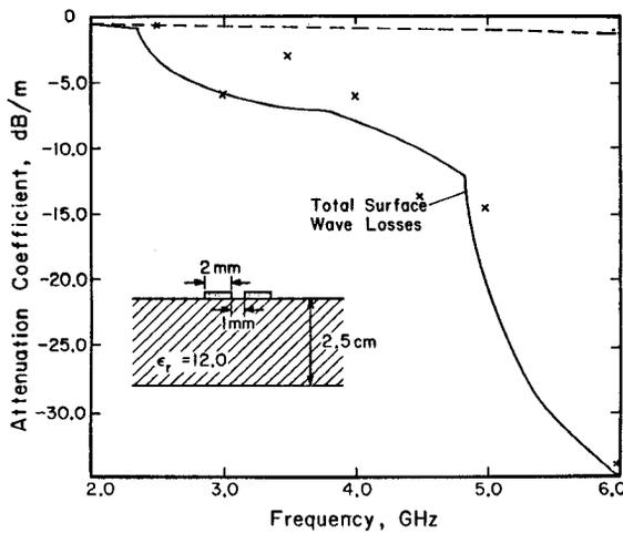
Fig. 8 (a) Measured losses, compared to theory for a two slot line.
