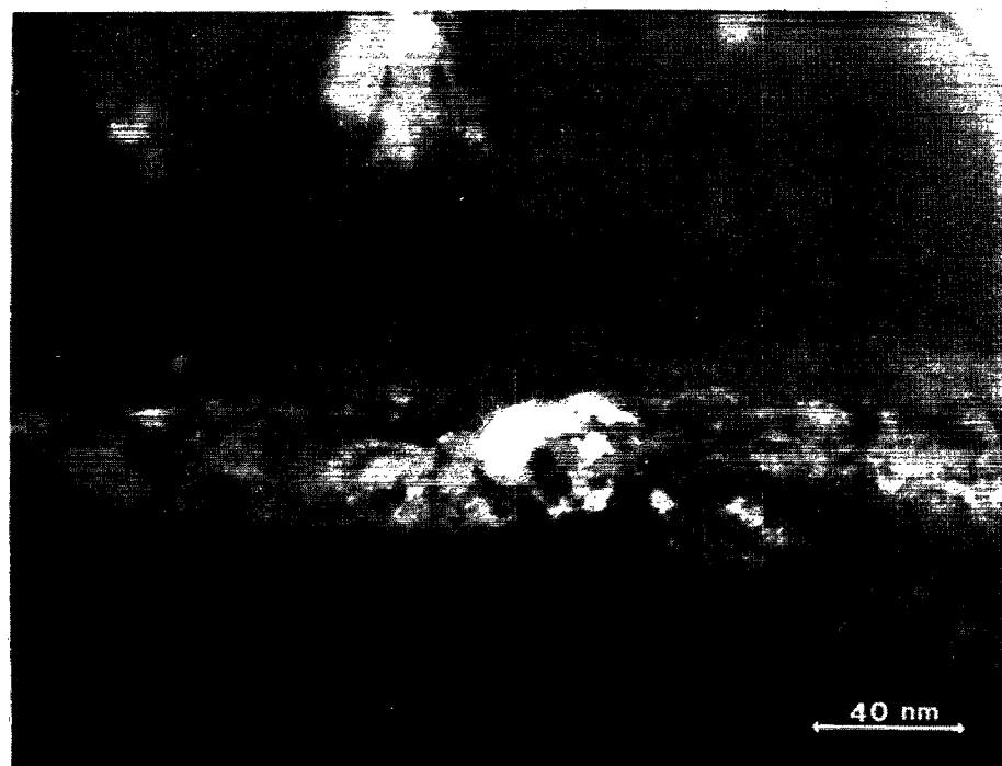
FIG. 3. (200) dark-field transmission electron micrograph of the same region shown in Fig. 2. The epigrown region is highlighted against that of the substrate due to the different deviation parameters induced by lattice strains in the epigrown layer.
