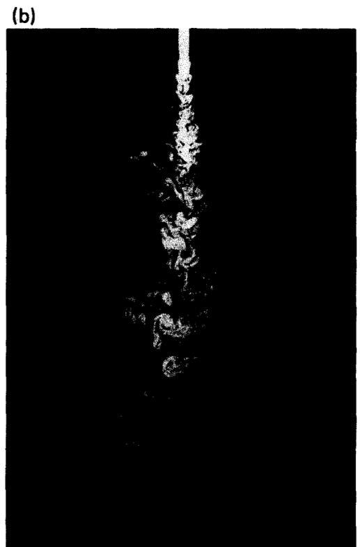
FIG. 5. Jet fluid field in the plane of symmetry of the jet ( $Re = 2500$ ,  $d = 0.75$  cm,  $0 < x/d < 35$ ). (a) Typical structure. (b) Evidence of spiral mode.
