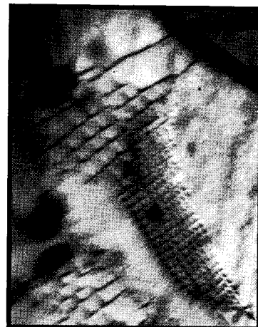
FIG. 1. Square dislocation network. \sim 80\,000\times .
