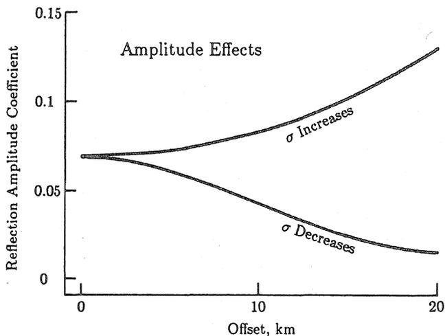
Figure 3. Comparison of reflection amplitudes at different offsets from an increase in Poisson's ratio from 0.347 to 0.392 and from a decrease from 0.347 to 0.292 at 12 km depth.
