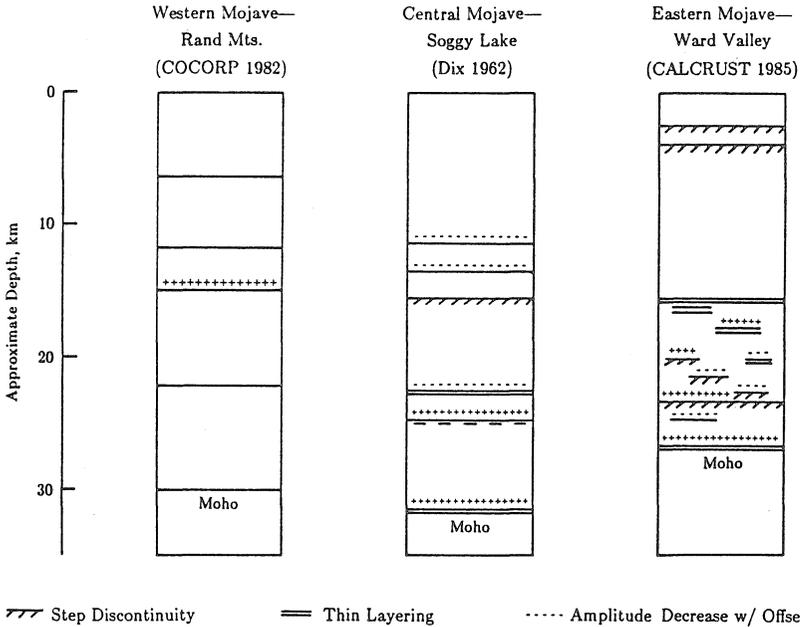
Figure 6. Generalized crustal columns showing the depths and character of major reflectors in 3 areas of the Mojave Desert. The physical nature of selected structures as derived from frequencies and amplitudes of multi-offset reflections are indicated. Increases or decreases of amplitude with offset are indicated by pluses or minuses above each reflector.
