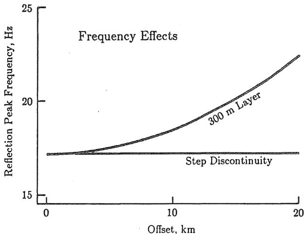
Figure 2. Comparison of the reflection peak frequency at different offsets from a thin layer and step discontinuity at 15 km depth.
