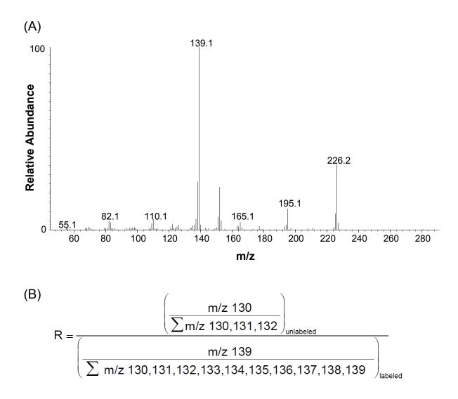
Additional Figure 1 Analyses of  $[{}^{13}C_{8}, {}^{15}N]IBA$  internal standards. (A) A full-scan mass spectrum showing ions generated from Me- $[{}^{13}C_{8}, {}^{15}N_{1}]IBA$ . (B) Equation showing the calculation of the R-value.
