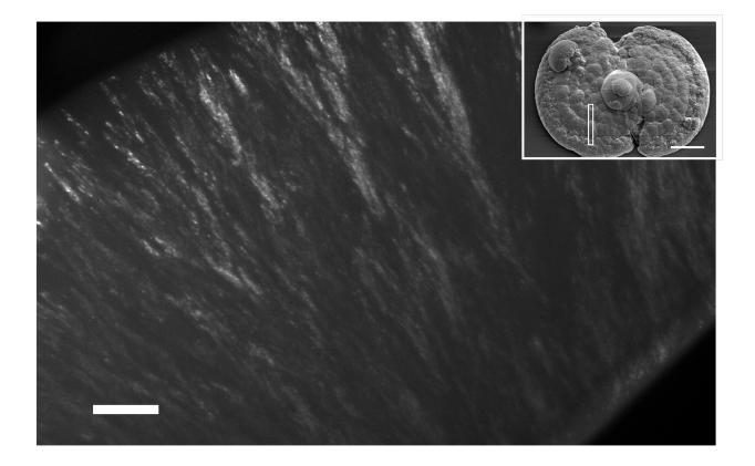
**Fig S1.** Cross-section of a botryoidal calcite nanoparticle aggregate (inset) that transforms from ACC under conditions with high Mg/Ca levels. TEM dark field image of FIB liftout shows high contrast (bright) regions that indicate nano-crystalline regions with similar orientations. Scale bar = 500 nm. Inset: SEM of botyroidal calcite aggregate with rectangular box that denotes the section of the sample where the FIB liftout was taken. Scale bar = 10 microns.
