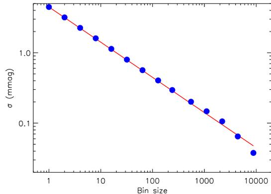
FIG. 4.— Scatter in the data (vertical axis) divided by the model binned by a number of bins (horizontal axis), averaged over the 14 transits and eclipses presented here. Red line is the extrapolation from the unbinned data by the inverse square root of the bin size.
