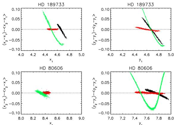
FIG. 1.— Comparison of the centroiding algorithms for HD 189733 versus M dwarf companion (top panels) and HD 80606 versus HD 80607 (bottom panels) in the  $x$ -direction (left panels) and  $y$  direction (right panels). The black dots are for the flux-weighted centroid, the red dots for the 2-D Gaussian centroid, and the green dots for the parabolic centroid. The HD 189733 data have been binned by 512 exposures (205 seconds), while the HD 80606 data have been binned by 4 exposures (56 seconds).
