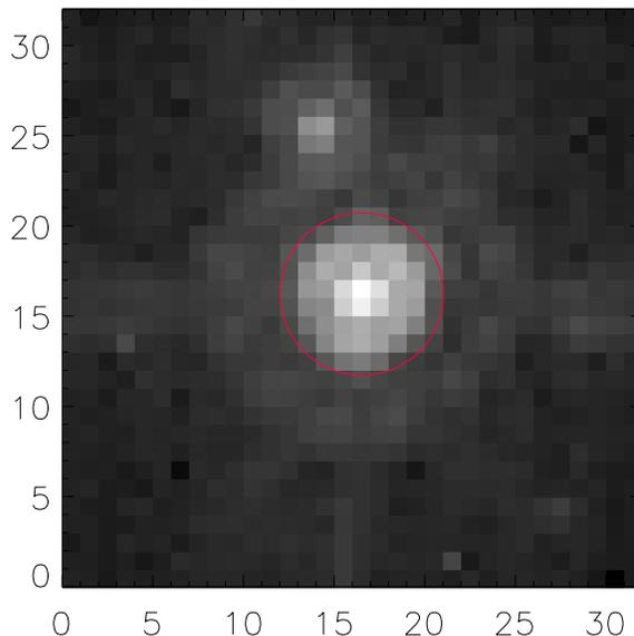
FIG. 2.— Logarithmic scaling of a median image from one of our observations; horizontal and vertical axes are pixels. White represents about 13,700 counts per pixel, while black is about 6 counts per pixel. The red circle is a 4.5 pixel radius aperture.
