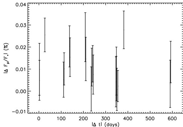
FIG. 15.— For each pair of eclipse observations, we show here the change in eclipse depth as a percent, versus the time between the observations. If the eclipse depths showed time-correlation—due to either astrophysical variability on some characteristic timescale or detector systematics—this plot would show a rise. The flat distribution is consistent with Gaussian variations at the level of a few percent.
