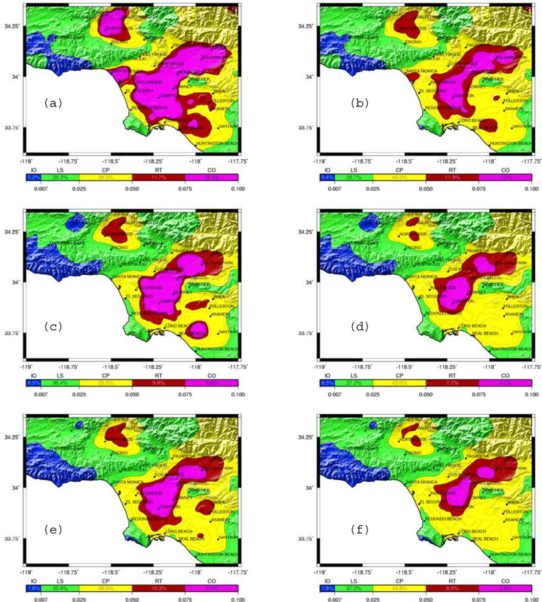
**Figure 4.** Maps of peak interstory drift for Building 1 with (a) susceptible and (b) perfect connections, Building 2 with (c) susceptible and (d) perfect connections, and Building 3 with (e) susceptible and (f) perfect connections. Color-coding corresponds to performance classification: Immediate Occupancy (IO); Life-Safety (LS); Collapse Prevention (CP); Red-Tagged (RT); Collapse (CO).
