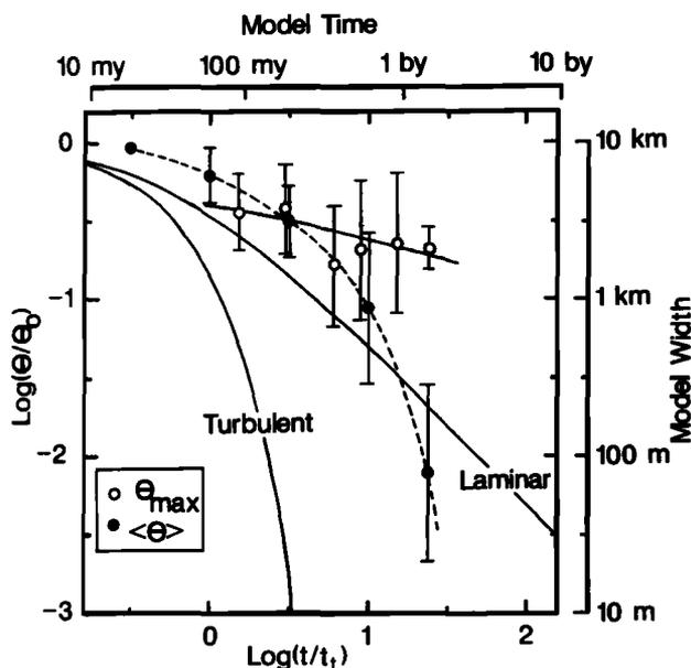
Fig. 3. Results of mixing calculations: the solid lines are the average width of the heterogeneity predicted by the simple laminar and turbulent mixing laws. The solid points are  $\langle \theta \rangle / \theta_0$  derived from the total lengths of material lines. The open points are for  $\theta_{\max} / \theta_0$  and were derived as shown in Figure 2, inset. The maximum sized heterogeneities mix slowly because they are laminarily mixed and occasionally unmixed within the interior of cells.
