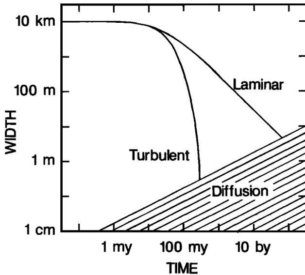
Fig. 1. Application of simple stirring laws to whole-mantle convection. The initial size of the heterogeneity is 10 km (= thickness of subducted crust). The shaded region is where chemical diffusion becomes important and is bound by the curve  $(\kappa t)^{1/2}$ , where  $\kappa = 10^{-13}$  cm<sup>2</sup>/s, an upper limit on the solid-state chemical diffusivity [Zindler and Hart, 1986].
