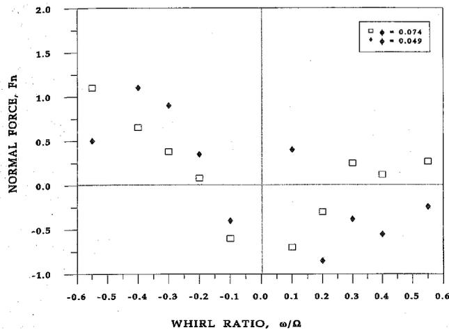
Fig. 12 Comparison of the normal force on the inducer at a cavitation number  $\sigma = 0.098$  for two flow coefficients. Uncertainty expressed as a standard deviation:  $F_n \pm 0.15$ ,  $\omega/\Omega \pm 0.001$ ,  $\phi \pm 0.00053$  and  $\sigma \pm 0.0039$ .
