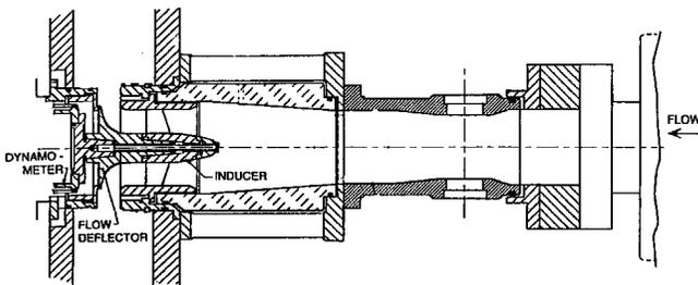
Fig. 1 (a) Schematic of inducer installation in the test facility
