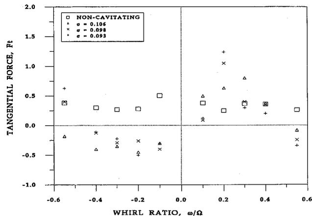
Fig. 5 Tangential force on the inducer at  $\phi = 0.074$  for various cavitation numbers. Uncertainty expressed as a standard deviation:  $F_t \pm 0.17$ ,  $\omega/\Omega \pm 0.001$ ,  $\phi \pm 0.00053$  and  $\sigma \pm 0.0039$ .
