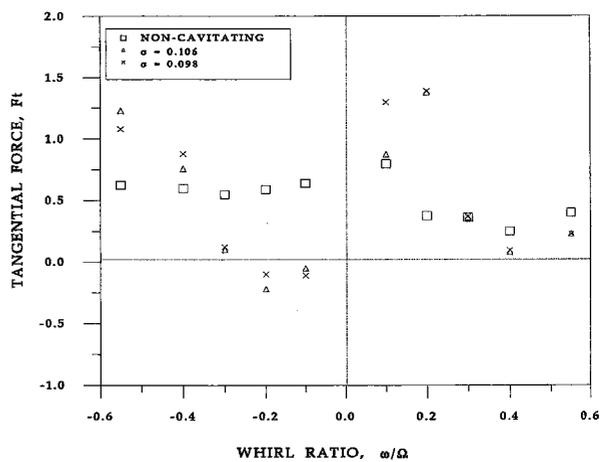
Fig. 6 Tangential force on the inducer at  $\phi = 0.049$  for various cavitation numbers. Uncertainty expressed as a standard deviation:  $F_t \pm 0.17$ ,  $\omega/\Omega \pm 0.001$ ,  $\phi \pm 0.00053$  and  $\sigma \pm 0.0039$ .
