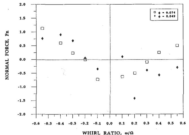
Fig. 11 Comparison of the normal force on the inducer at a cavitation number  $\sigma = 0.106$  for two flow coefficients. Uncertainty expressed as a standard deviation:  $F_n \pm 0.15$ ,  $\omega/\Omega \pm 0.001$ ,  $\phi \pm 0.00053$  and  $\sigma \pm 0.0039$ .
