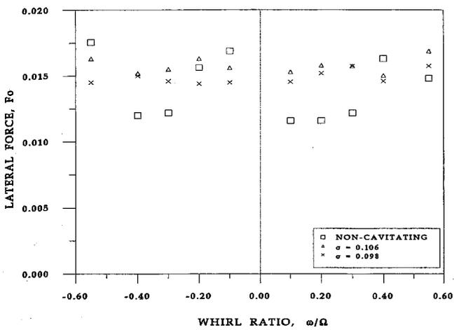
Fig. 4 Lateral force on the inducer at  $\phi = 0.049$  for various cavitation numbers. Uncertainty expressed as a standard deviation:  $\|F_0\| \pm 0.00091$ ,  $\omega/\Omega \pm 0.001$ ,  $\phi \pm 0.00053$  and  $\sigma \pm 0.0039$ .
