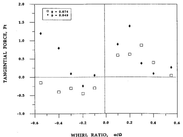
Fig. 7 Comparison of the tangential force on the inducer at a cavitation number  $\sigma = 0.106$  for two flow coefficients. Uncertainty expressed as a standard deviation:  $F_t \pm 0.17$ ,  $\omega/\Omega \pm 0.001$ ,  $\phi \pm 0.00053$  and  $\sigma \pm 0.0039$ .
