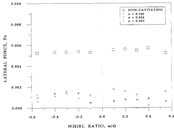
Fig. 3 Lateral force on the inducer at  $\phi = 0.074$  for various cavitation numbers. Uncertainty expressed as a standard deviation:  $\|F_o\| \pm 0.00091$ ,  $\omega/\Omega \pm 0.001$ ,  $\phi \pm 0.00053$  and  $\sigma \pm 0.0039$ .
