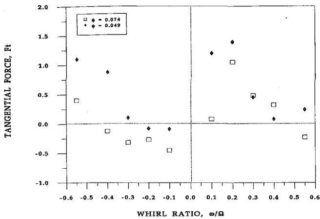
Fig. 8 Comparison of the tangential force on the inducer at a cavitation number  $\sigma = 0.098$  for two flow coefficients. Uncertainty expressed as a standard deviation:  $F_t \pm 0.17$ ,  $\omega/\Omega \pm 0.001$ ,  $\phi \pm 0.00053$  and  $\sigma \pm 0.0039$ .
