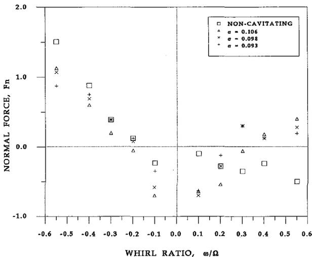
Fig. 9 Normal forces at flow coefficient  $\phi = 0.074$  for various cavitation numbers. Uncertainty expressed as a standard deviation:  $F_n \pm 0.15$ ,  $\omega/\Omega \pm 0.001$ ,  $\phi \pm 0.00053$  and  $\sigma \pm 0.0039$ .
