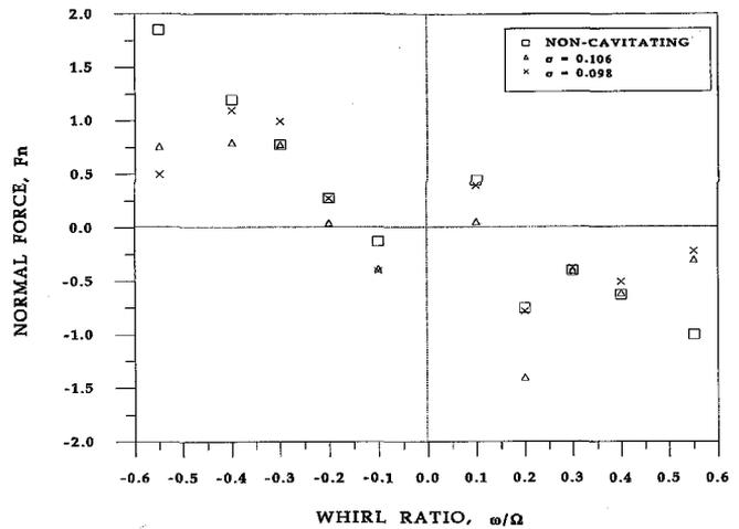
Fig. 10 Normal forces at flow coefficient  $\phi = 0.049$  for various cavitation numbers. Uncertainty expressed as a standard deviation:  $F_n \pm 0.15$ ,  $\omega/\Omega \pm 0.001$ ,  $\phi \pm 0.00053$  and  $\sigma \pm 0.0039$ .
