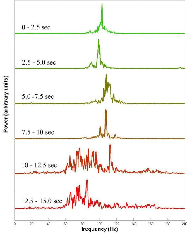
FIG. 4: Spectra of 2.5-second clips of a booming event at Dumont Dunes show that the frequency of the booming changes over the duration of a slide.
