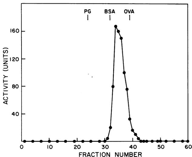
Fig. 6. Sucrose sedimentation velocity. 70  $\mu$ l containing 3,000 units of Fraction V and marker proteins was sedimented through a preformed 5-20% linear sucrose gradient in 0.5 M KCl, 0.02 M potassium phosphate (pH 7.3), 1 mM EDTA, and 0.1 mM PMSF. Centrifugation was in a SW50.1 rotor at 40,000 rpm for 22 hours at 4 $^{\circ}$ . Fractions of 84  $\mu$ l were collected at 4 $^{\circ}$ . The markers were canine serum plasminogen, BSA, and ovalbumin.
