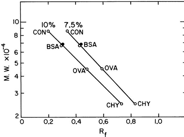
Fig. 5. The molecular weight of the denatured and reduced nicking-closing enzyme was determined by comparing its electrophoretic mobility ( $R_f$ ) with those of protein standards, conalbumin (CON), BSA, ovalbumin (OVA), chymotrypsinogen (CHY).
