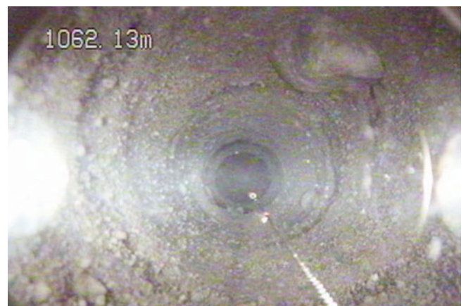
Fig. 15. Large smooth rock partly embedded in rough borehole wall 1 m above base of ice.
