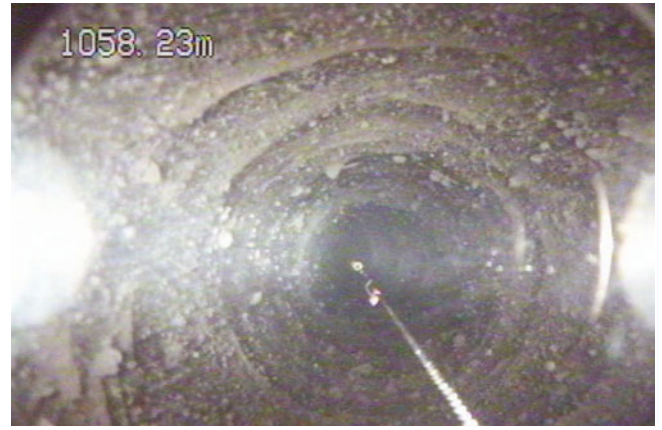
Fig. 14. Elevated debris content, with rocks sticking out from a rough borehole wall.
