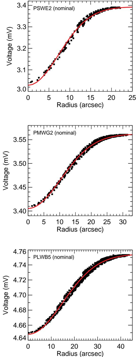
**Figure 8.** Examples of the signal measured from Neptune in the fine scan observation 1342186522, which used the nominal voltage bias setting. The red line shows the best fitting function to the data. Data falling within the background annulus were included in the fit but are not included in this plot.
