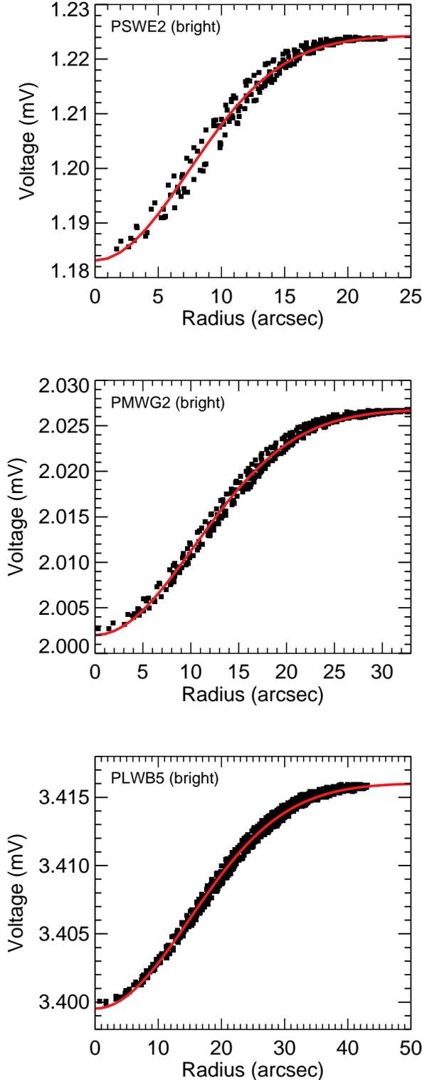
**Figure 9.** Examples of the signal measured from Neptune in the fine scan observation 1342187438, which used the bright source bias setting. The red line shows the best fitting function to the data. Data falling within the background annulus were included in the fit but are not included in this plot.
