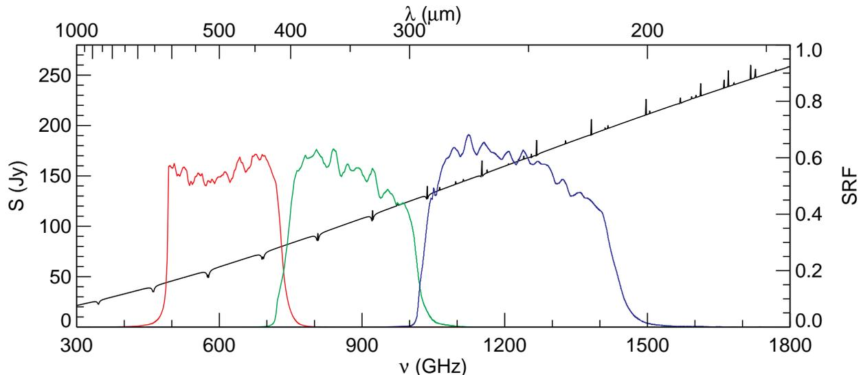
**Figure 2.** The model spectrum of Neptune on OD 168 (29 Oct 2009) in black along with the SRFs of the three SPIRE photometer bands (from <ftp://ftp.science.nasa.gov/pub/hsc-calibration/SPIRE/PHOT/Filters/>), with the blue, green, and red curves corresponding to the 250, 350, and 500  $\mu\text{m}$  bands, respectively.
