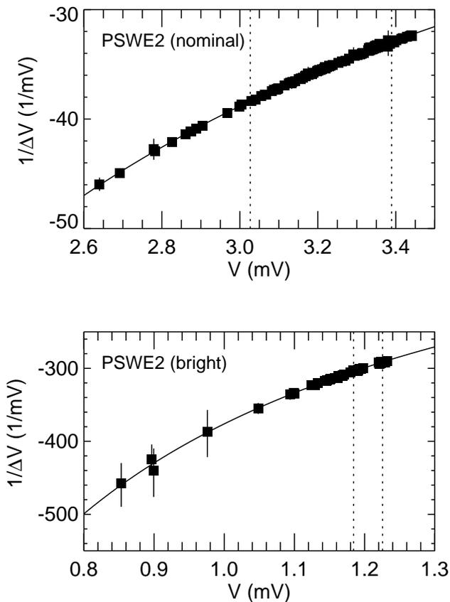
**Figure 7.** PCal flash data for PSWE2. Data are shown for both bias modes. Lower voltages correspond to viewing brighter regions of sky. The solid line shows the function described by Equation 3 that was fitted to the data. The dotted lines show the mean peak and background signal measured for Neptune in the fine scan observations described in Section 6.
