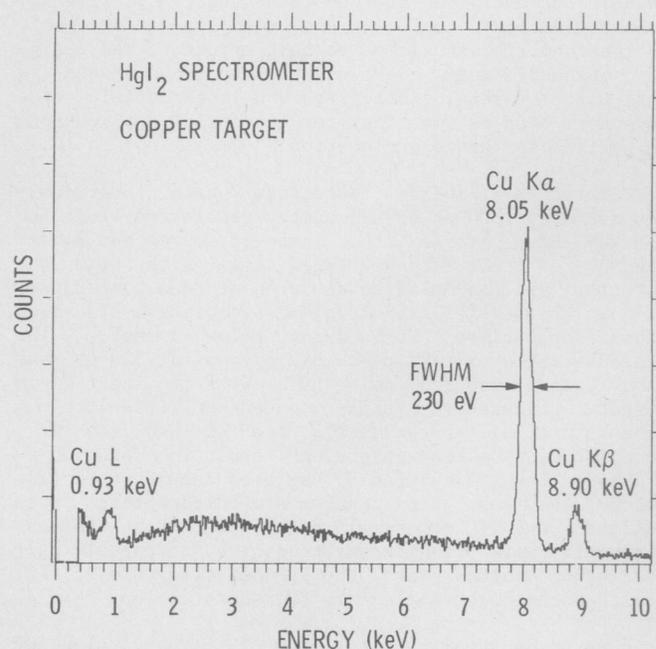
Figure 2. X-ray spectrum obtained from copper target
