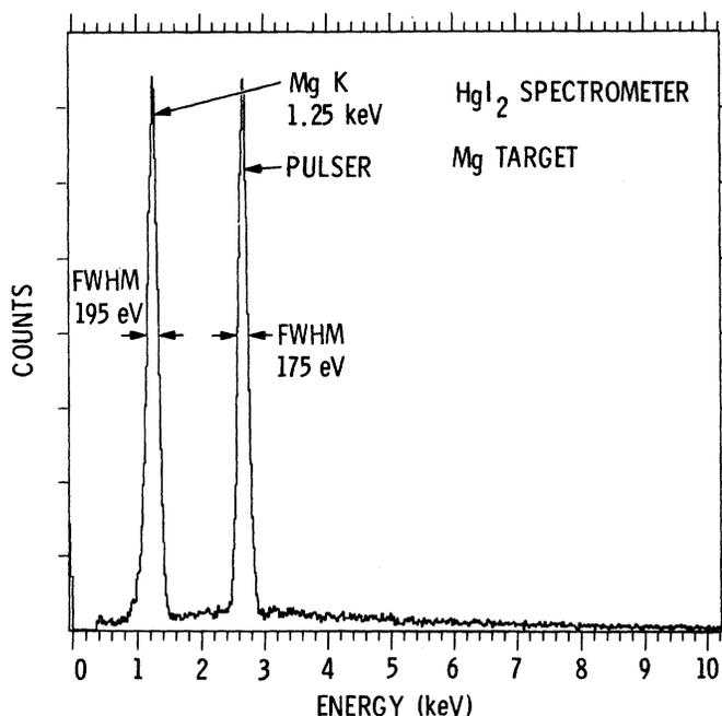
Figure 4. X-ray spectrum obtained from magnesium target. (Electronic pulser indicates system noise)
