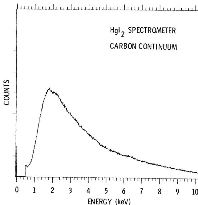
Figure 5. X-ray spectrum obtained from carbon target
