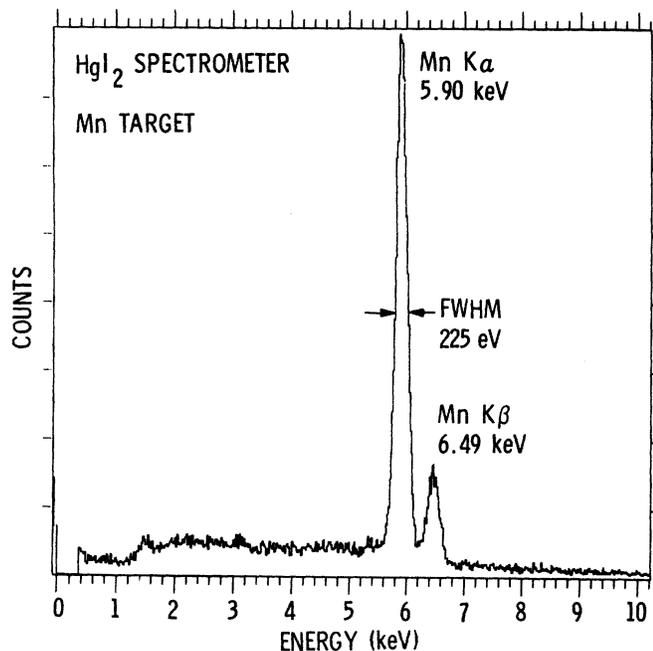
Figure 3. X-ray spectrum obtained from manganese target
