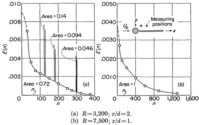
FIGURE 22.—Effect of downstream plate on wake frequencies.
