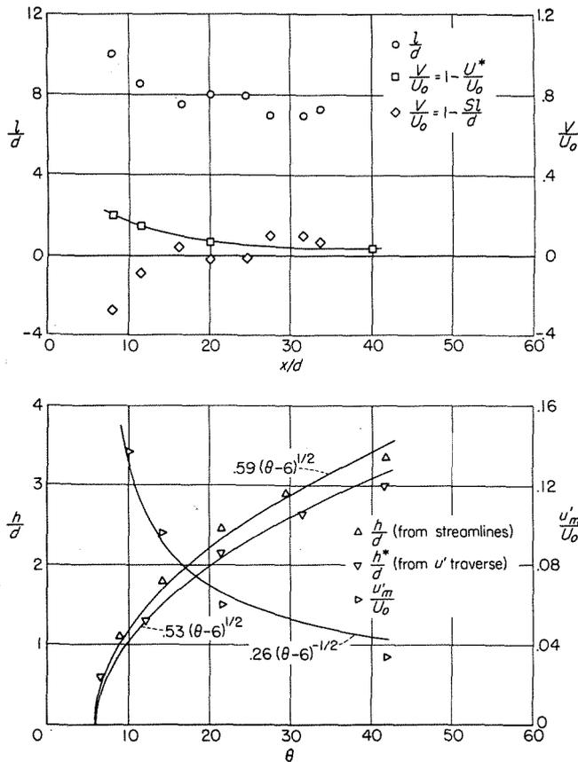
FIGURE 21.—Vortex-street geometry. Calculated from data in reference 11.
