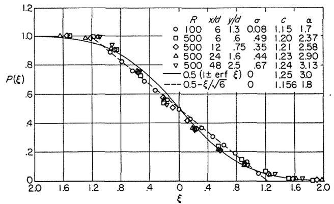
FIGURE 19.—Distribution functions.  $d=0.190$  centimeter.
