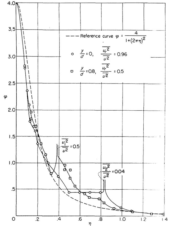
FIGURE 16.—Spectra at 12 diameters.  $d=0.190$  centimeter;  $R=500$ ;  $n_1=430$ .
