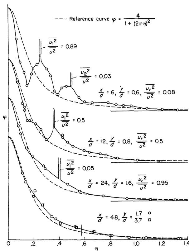
FIGURE 14.—Downstream development of spectrum.  $d=0.190$  centimeter;  $R=500$ ;  $n_1=440$ .
