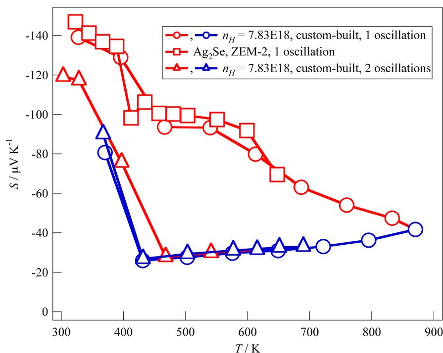
Figure S7: Effects of including an additional oscillation during measurement of the Seebeck coefficient of ingot samples of  $\text{Ag}_2\text{Se}$ . Red curves are heating data, blue curves are cooling data.
