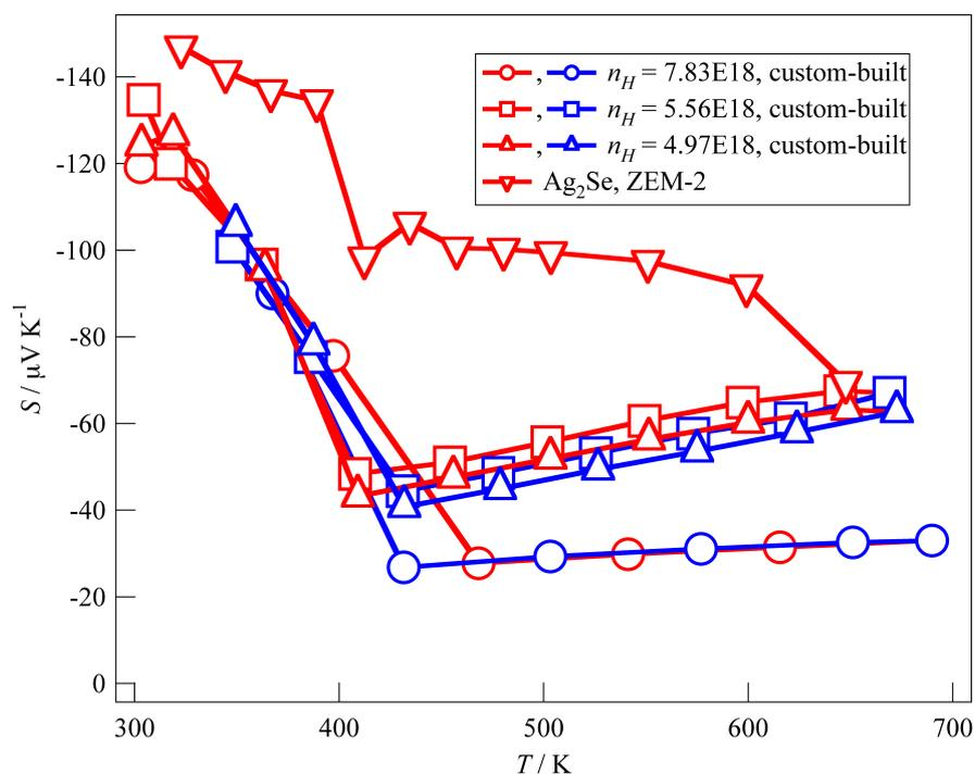
Figure S6: Seebeck coefficient of disks sliced from ingots. Red curves are heating data, blue curves are cooling data.
