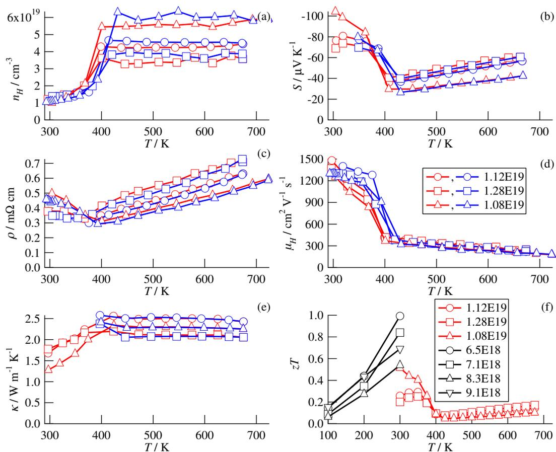
Figure S3: Transport properties of hot-pressed samples. Red curves are heating data, blue curves are cooling data. Black curves are from Aliev.<sup>[1]</sup>
