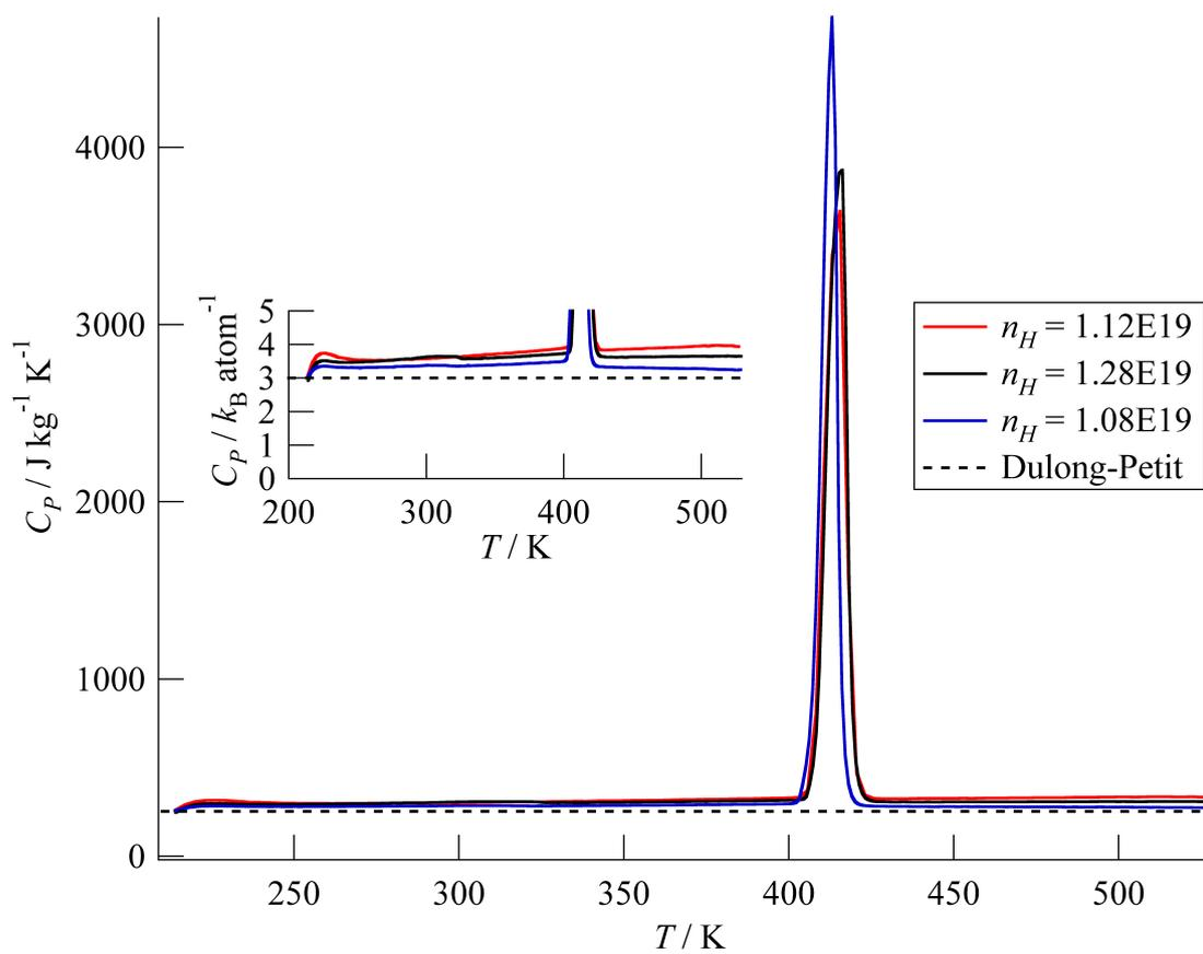
Figure S1: Heat capacity of hot-pressed samples
