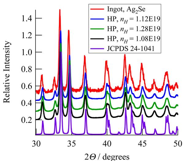
Figure S8: XRD scans of  $\text{Ag}_{2+x}\text{Se}$  at room temperature
