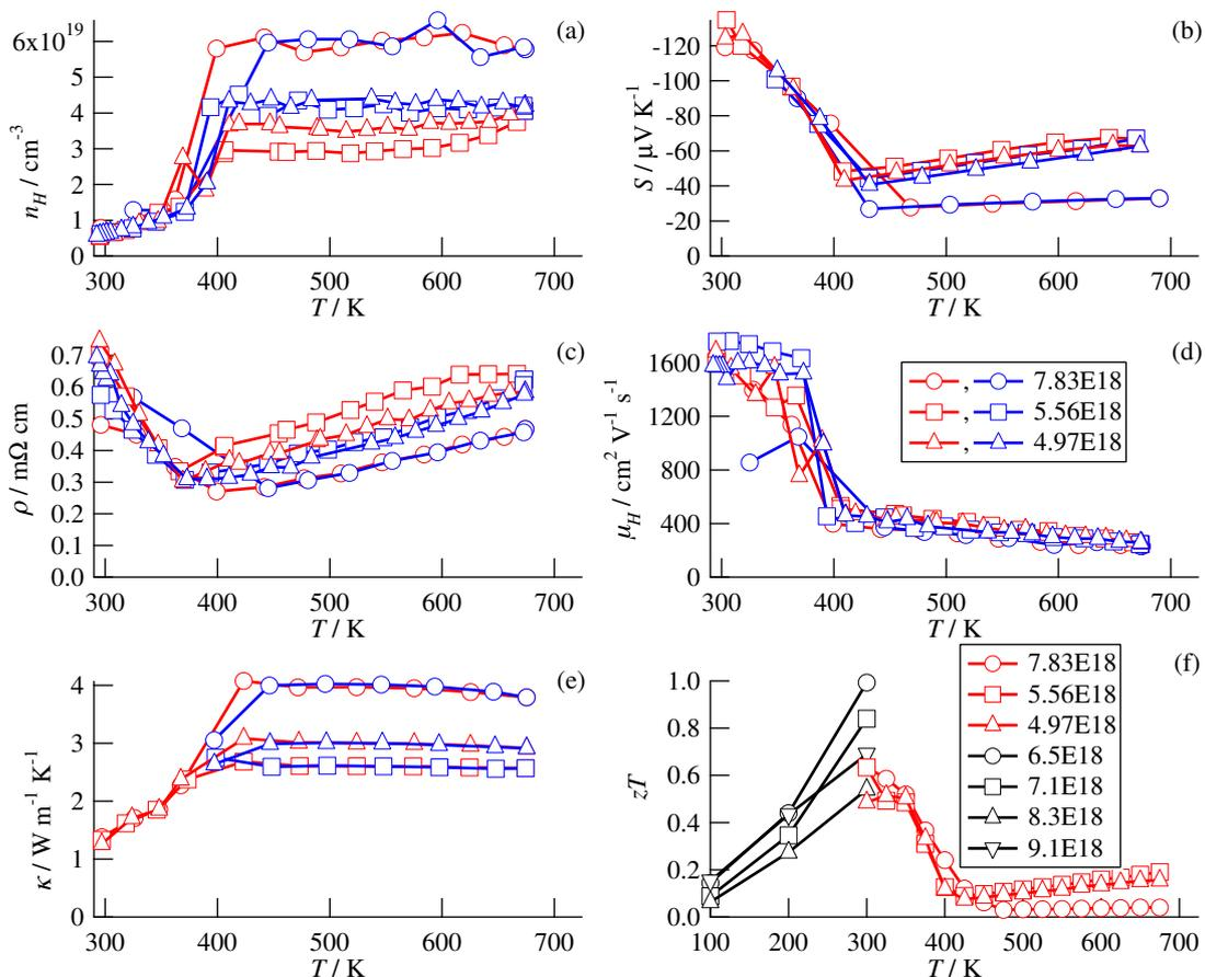
Figure S4: Transport properties of ingot samples. Red curves are heating data, blue curves are cooling data. Black curves are from Aliev.<sup>[1]</sup>
