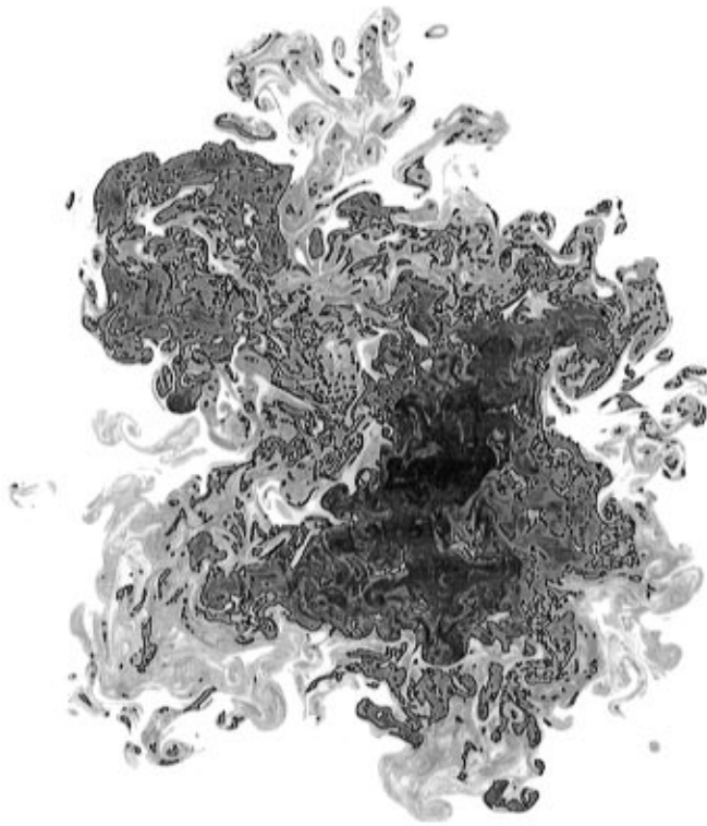
FIG. 4. Level set of jet-fluid concentration in the far field ( z/d_j = 275 ) of a liquid-phase turbulent jet at Re \approx 9 \times 10^3 .
