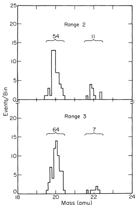
FIG. 3.—Mass histograms of range 2 and range 3 neon events. The  $^{22}\text{Ne}$  energy intervals are 11–15 and 15–26 MeV per nucleon, while those for  $^{20}\text{Ne}$  are  $\sim 6\%$  higher.
