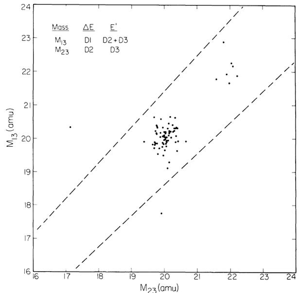
FIG. 2.—Comparison of mass measurements for range 3 neon events. Events outside the dashed lines were rejected.
