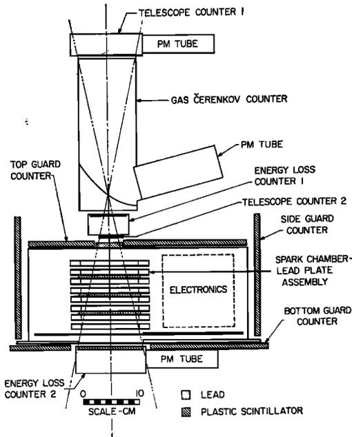
Fig. 1. Cross section of the detector system.
