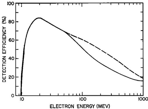
Fig. 2. Electron detection efficiency versus kinetic energy at the top of the detector. Solid curve indicates efficiency with all selection criteria included; dashed curve, efficiency with fourth criterion ignored.
