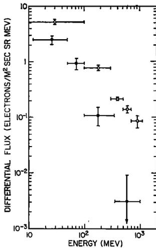
Fig. 8. Differential kinetic energy spectrum of splash albedo electrons. Solid circles represent present experiment, Fort Churchill, Canada; open circles, experiment of Verma [1967a], Palestine, Texas.
