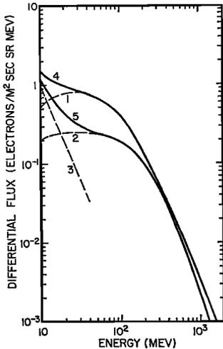
Fig. 3. Kinetic energy spectrum of atmospheric secondary electrons at 2-g/cm<sup>2</sup> atmospheric depth. Curve 1 represents electrons from nuclear interactions [Perola and Scarsi, 1966]; curve 2, electrons from nuclear interactions [Verma, 1967b]; curve 3, knock-on electrons; curve 4, sum of curves 1 and 3; curve 5, sum of curves 2 and 3.
