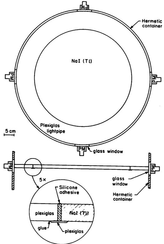
Figure 1. Schematic diagram showing mounting of the scintillator and the viewing system with four photomultipliers.
