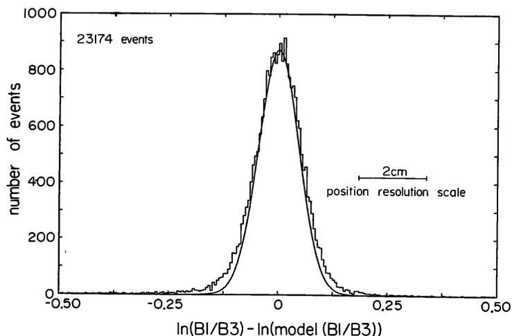
**Figure 4.** Deviation of response from that expected for particles near the center of the counter.
