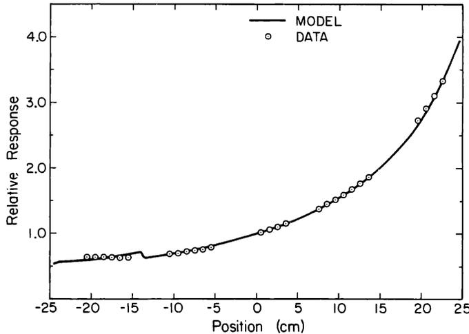
Figure 3. Relative response for a single photomultiplier as a function of position along a diameter of the disc. The phototube is placed at about +40 cm at the outside of the plexiglas lightpipe.
