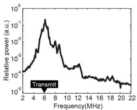
**Supplementary Figure S3. Harmonic ultrasound response of *Ana* GVs.** Power spectrum of signal backscattered from OD 2.0 *Ana* GVs in response to 6 MHz ultrasound pulses (peak amplitude 98 kPa). Each point represents an average of 16 measurements.
