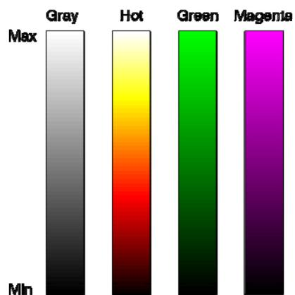
**Supplementary Figure S9. Colour maps used in ultrasound images.** Gray, Hot, Green and Magenta colour maps as used in Figs. 1-4 in the main text and Supplementary Figs. S1, S2 and S4. The scales are linear between Min and Max. The colour map used and the values of Min and Max are defined for each image in Supplementary Table S1. The colour maps Gray and Hot are standard in MATLAB. Green and Magenta were prepared by replacing the color white with either green or magenta in the Gray color map.
